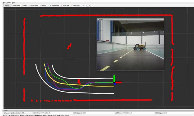
Figure 22. Planning results for the different algorithms.
