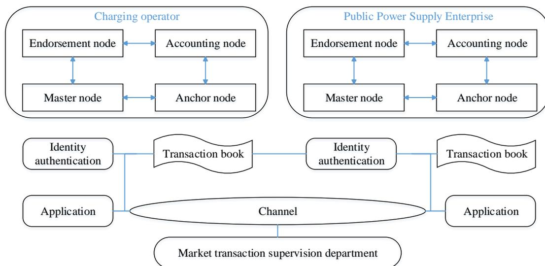
Figure 1. Network structure of electric vehicle charging transaction model.
