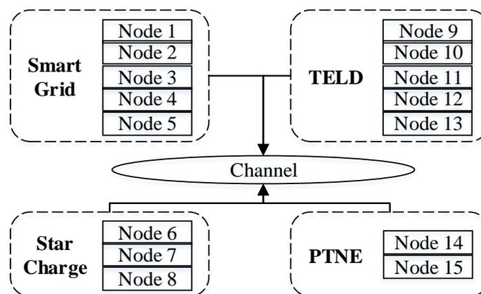
**Figure 4.** Network topology for charging transaction.
