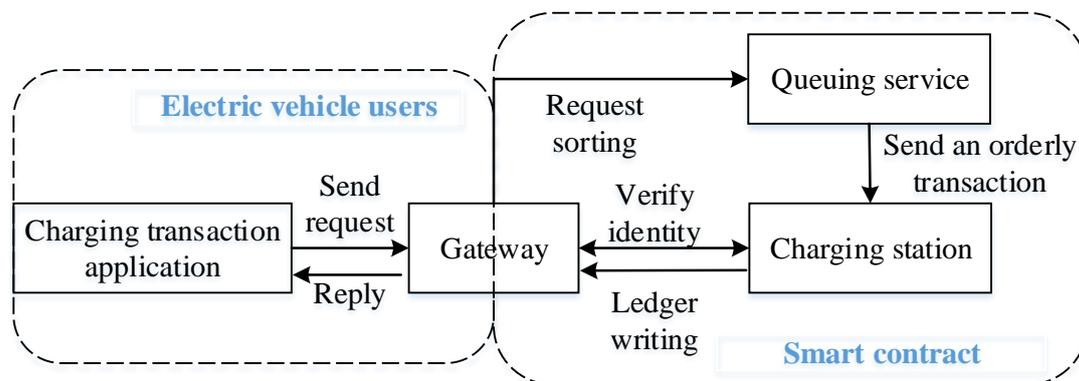
Figure 3. Operation process of electric vehicle charging transaction model.
