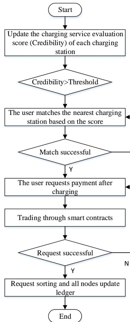
**Figure 5.** Flow chart of electric vehicle charging transaction model.
