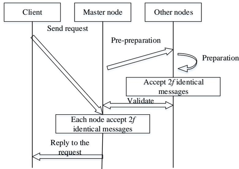
Figure 2. Sequence diagram of PBFT consensus algorithm.
