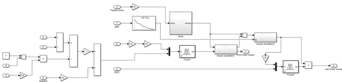
**Figure 13.** Torque distribution control strategy based on fuzzy control.
