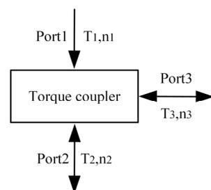
**Figure 2.** Torque coupler.
