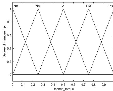
Figure 9. Affiliation function of desired torque.
