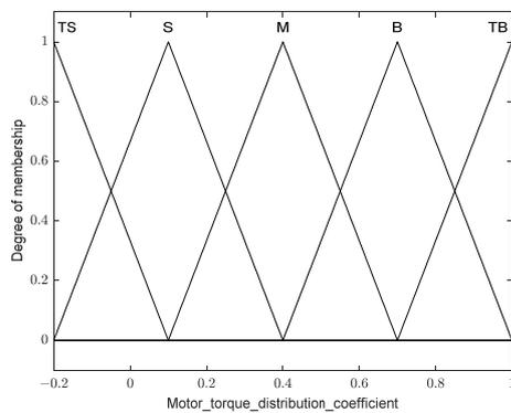
Figure 11. Affiliation function of motor torque distribution coefficient.
