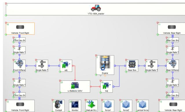
**Figure 12.** Hybrid four-wheel drive tractor vehicle model.
