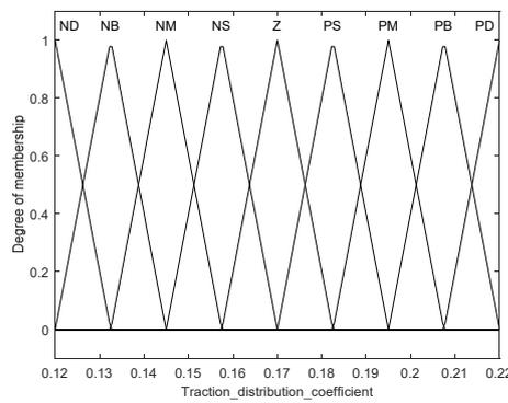
Figure 7. Affiliation function of tractive force distribution coefficient.
