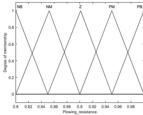
Figure 5. Affiliation function of plowing resistance.
