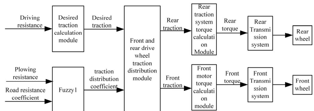
**Figure 3.** Control strategy for torque distribution of front- and rear-drive wheels based on fuzzy control.
