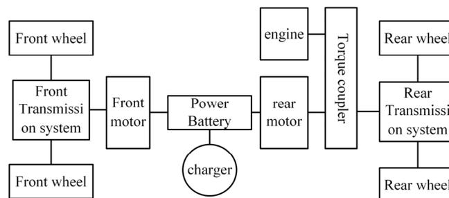
**Figure 1.** Hybrid four-wheel drive tractor power system.
