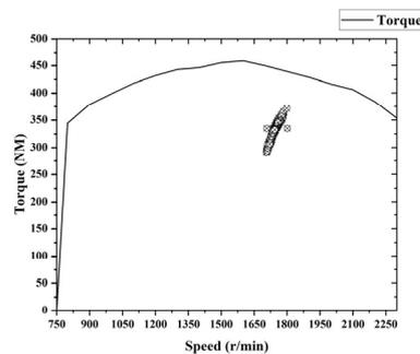
**Figure 21.** Engine working point distribution map.
