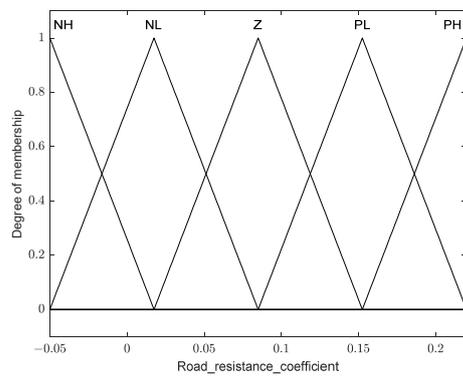
Figure 6. Affiliation function of road resistance coefficient.
