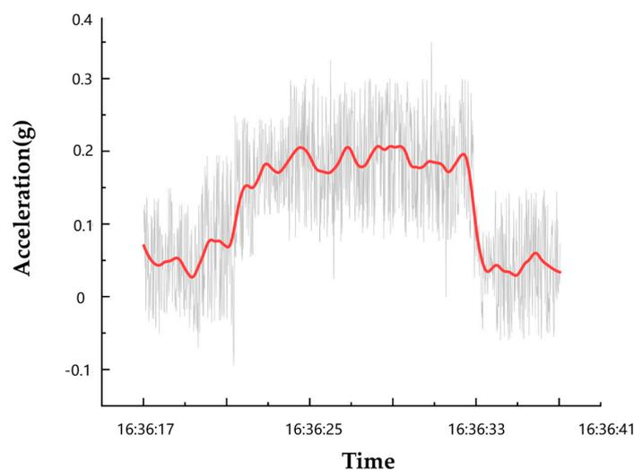
**Figure 7.** Acceleration data of the vehicle in the Y-axis direction. The gray lines are the raw data, and the red line is the result of filtering.
