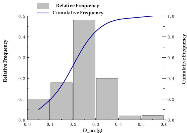
**Figure 9.** Frequency statistics chart of vehicle lateral acceleration data.
