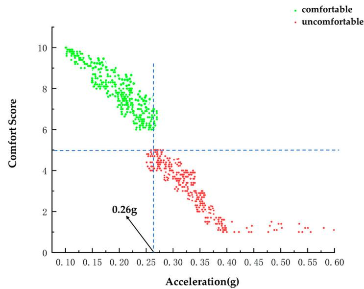
**Figure 11.** Visualization of scatter plots of vehicle lateral acceleration and passenger comfort scores and comfort status domain boundaries.
