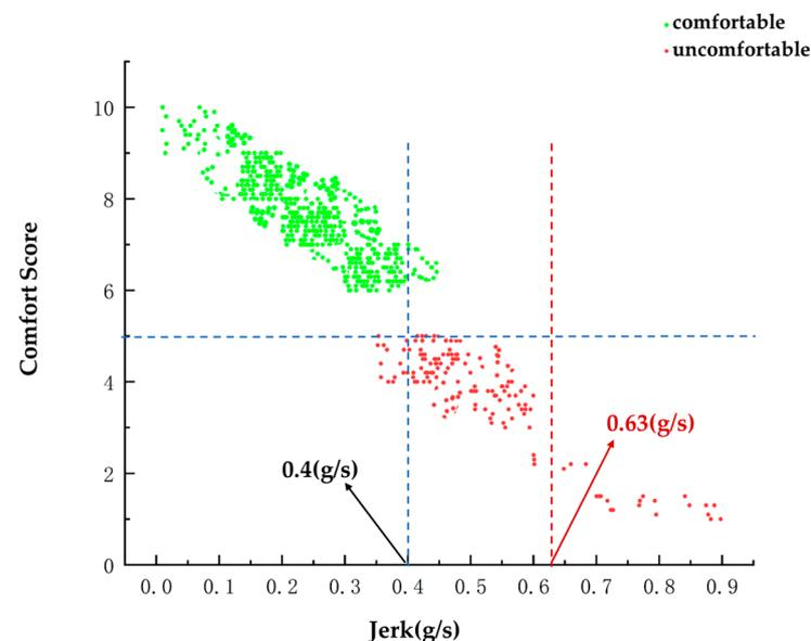
**Figure 14.** Visualization of scatter plots of vehicle lateral jerk and passenger comfort scores and extreme status domain boundaries.
