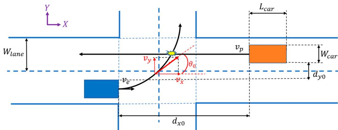
**Figure 16.** Vehicle kinematic model and related parameters. The blue rectangle represents the left-turning vehicle (SV), and the orange rectangle represents the vehicle going straight (POV).
