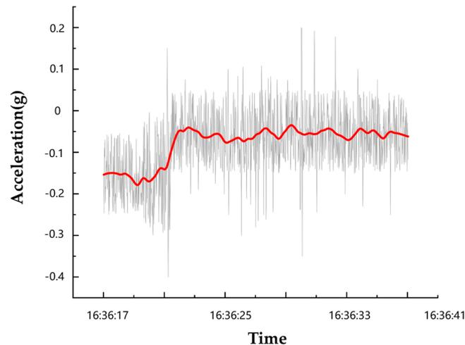
**Figure 6.** Acceleration data of the vehicle in the X-axis direction. The gray lines are the raw data, and the red line is the result of filtering.
