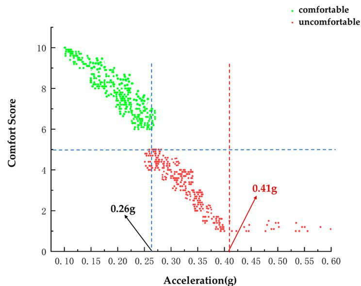
**Figure 13.** Visualization of scatter plots of vehicle lateral acceleration and passenger comfort scores and extreme status domain boundaries.
