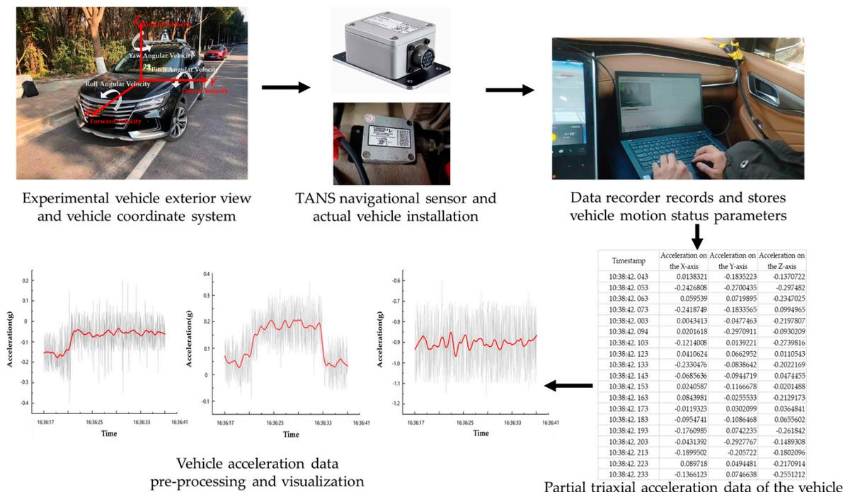
**Figure 4.** Experimental data acquisition and processing process. The gray lines are the raw data, and the red line is the result of filtering.
