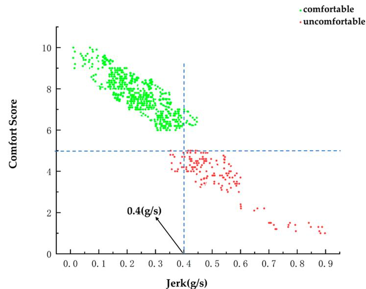
**Figure 12.** Visualization of scatter plots of vehicle lateral jerk and passenger comfort scores and comfort status domain boundaries.
