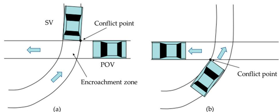
**Figure 17.** Analysis of main conflict points. (a) represents the SV crossing the intersection before the POV; (b) represents the SV crossing the intersection after the POV.
