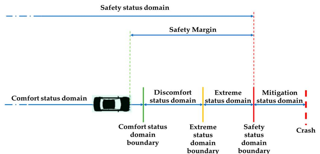
**Figure 2.** Schematic diagram of each status domain and boundary.
