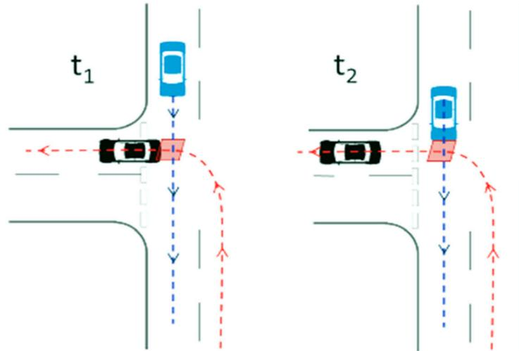
**Figure 15.** Illustration of the two moments in time used in the calculation of PET when one vehicle turns left (the black vehicle, SV, its trajectory is shown by the red dashed line) in front of an oncoming vehicle (the blue vehicle, POV, its trajectory is shown by the blue dashed line) with the right-of-way. The red rhombus is the encroachment zone.  $PET = t_2 - t_1$  [20].
