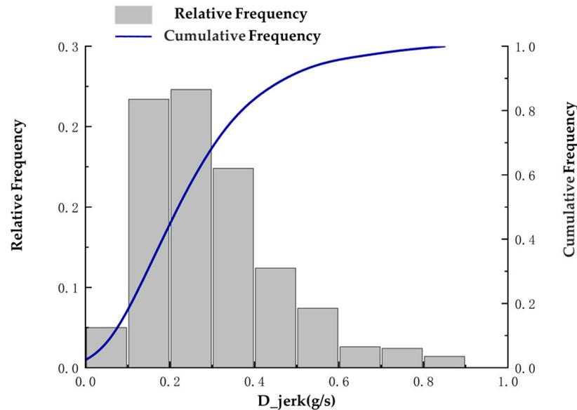
Figure 10. Frequency statistics chart of vehicle lateral jerk data.
