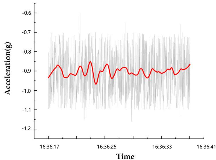
**Figure 8.** Acceleration data of the vehicle in the Z-axis direction. The gray lines are the raw data, and the red line is the result of filtering.
