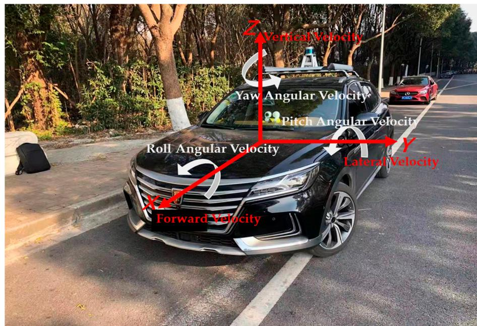
**Figure 3.** Experimental vehicle exterior view and vehicle coordinate system.
