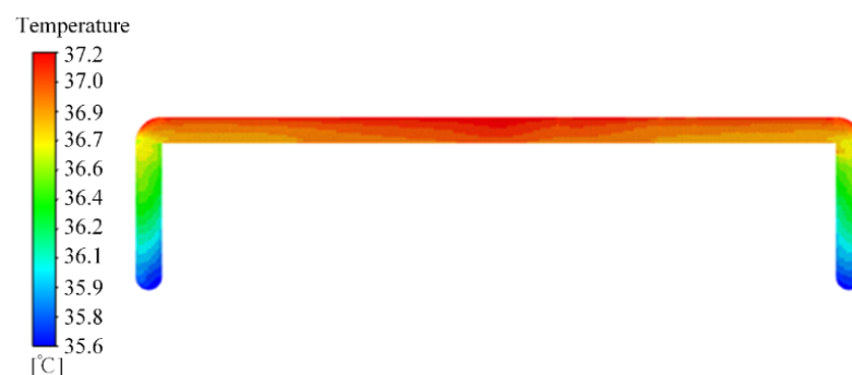
Figure 3. Cloud diagram of temperature distribution of rotating heat pipe.
