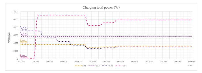
Figure 8. Total charging power per EV, during GridShield intervention.
