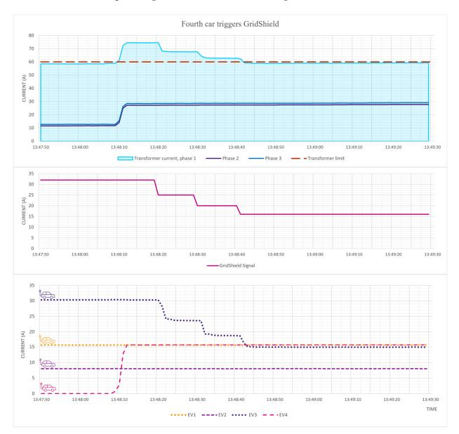
**Figure 6.** Transformer current, GridShield signal, and EV charging when an additional EV overloads the system.
