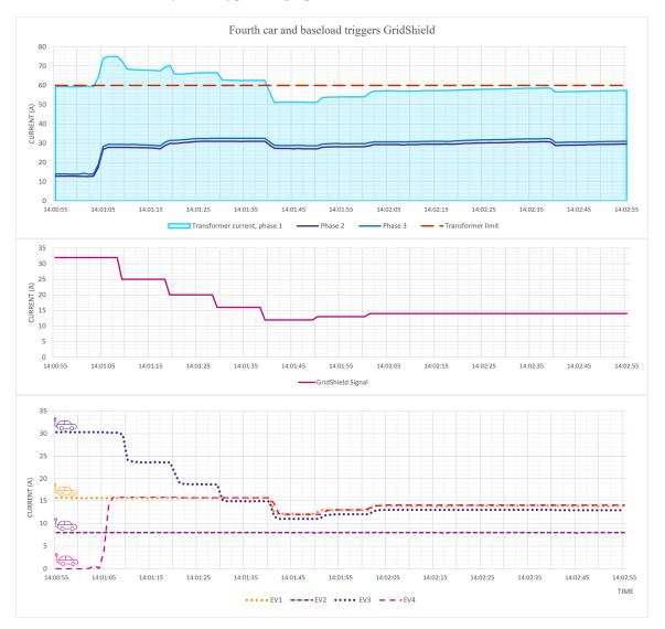
Figure 7. Transformer current, GridShield signal, and EV charging (ampere).
