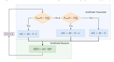
**Figure 4.** Block diagram of the AIMD GridShield algorithm. Blue: sender-side implementation. Green: receiver-side implementation. Adapted from [21].
