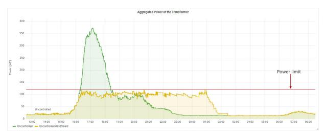
Figure 5. Digital twin simulation of a Dutch neighborhood with 80 EVs.
