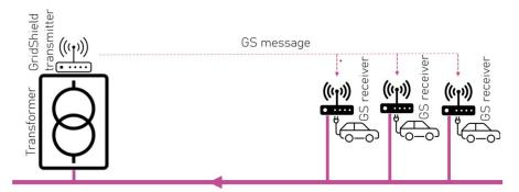
Figure 3. Schematic overview of the GridShield transmitter and receiver [19].
