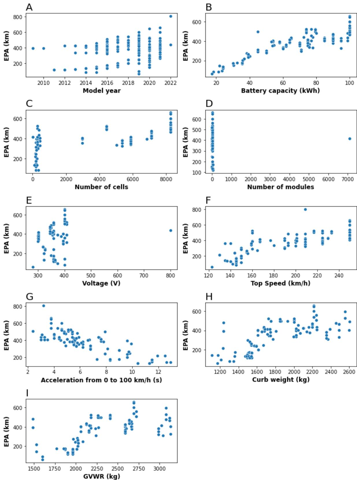
**Figure 4.** Plots of independent variables against EPA range, where the independent variables are (A) model year, (B) battery capacity (in KWh), (C) number of battery cells in an EV, (D) number of battery modules, (E) EV battery pack voltage, (F) EV top speed (in km/h), (G) EV acceleration from 0 to 100 km/h (in s), (H) EV curb weight (in kg), and (I) gross vehicle weight rating (in kg).
