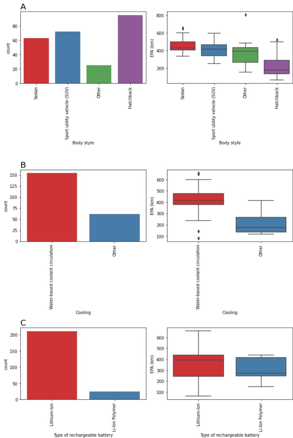
**Figure 6.** Histograms and boxplots of (A) EV body style, (B) battery cooling mechanism, and (C) type of lithium-ion battery used. The histograms plot the frequency (referred to as the count) of data points against the qualitative independent variables. Boxplots display the average and quartiles of the EPA range against the qualitative independent variables.
