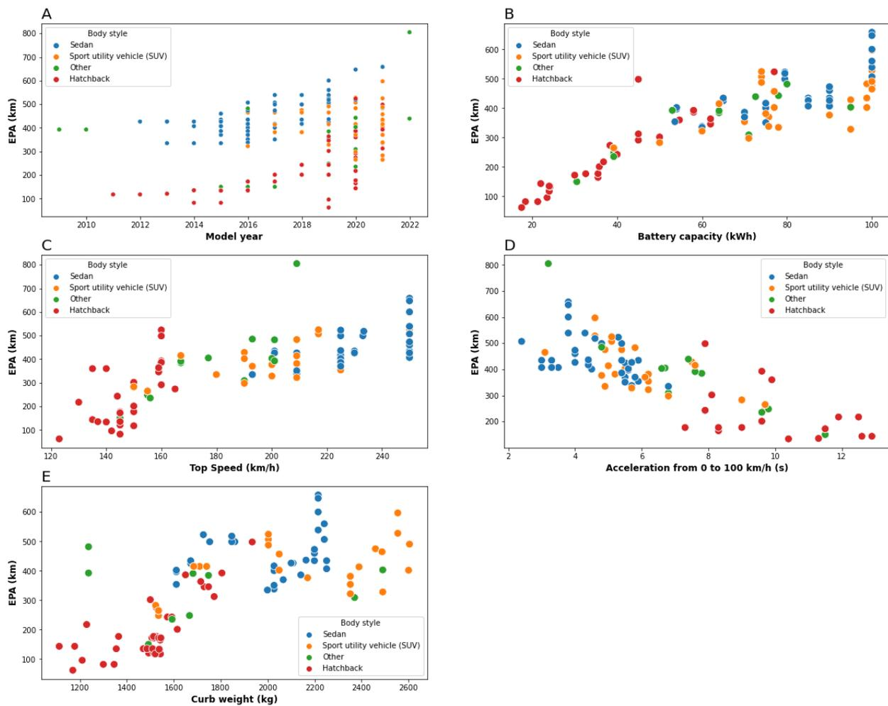
**Figure 5.** Scatter plot of independent variables, (A) EV model year, (B) battery capacity (in kWh), (C) top speed, (D) acceleration from 0 to 100 km/h (in s), and (E) EV curb weight (in kg), with EPA range, with scatter points colored differently based on EV body style.
