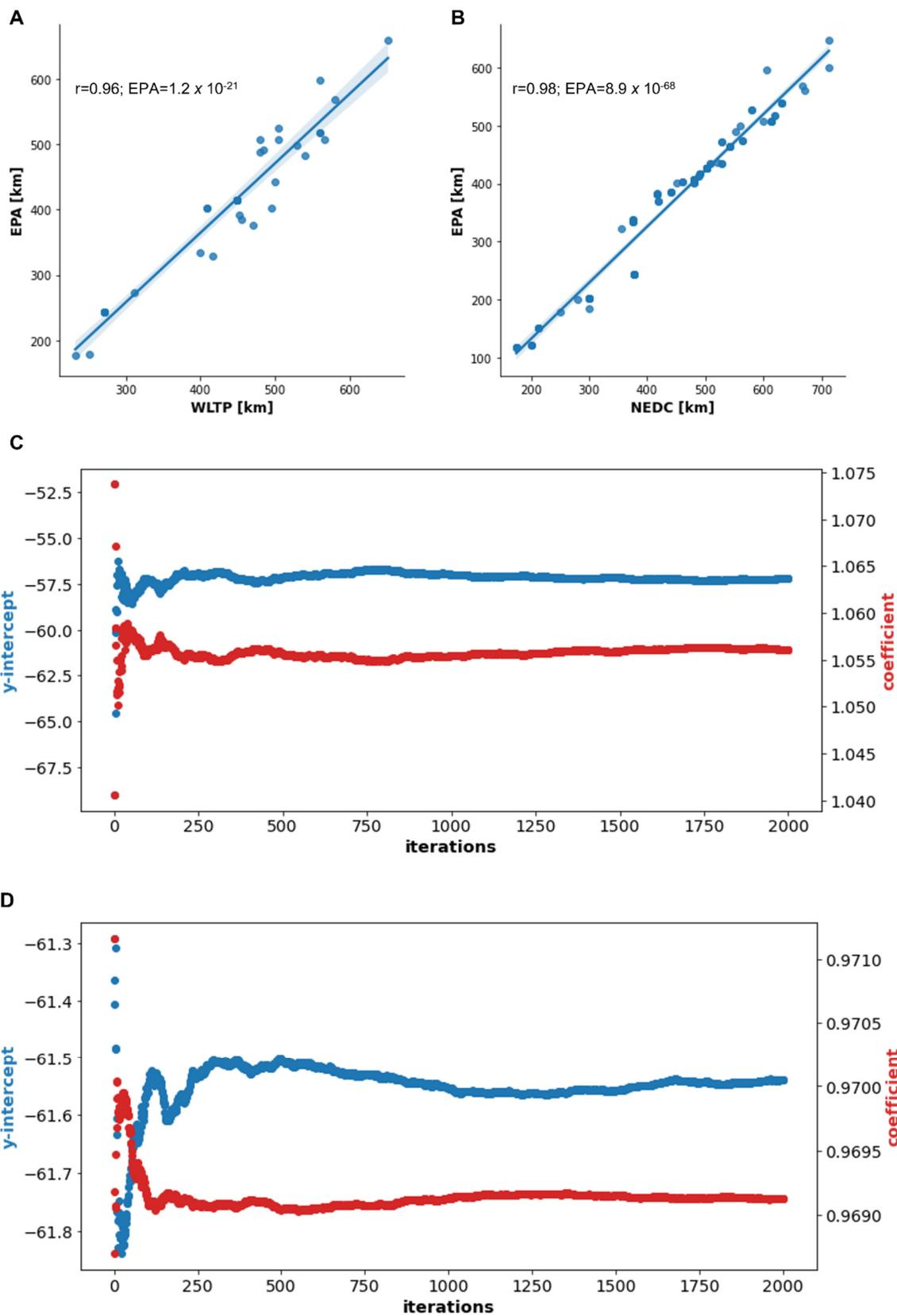
**Figure 3.** A plot, along with the lines of best fit and Pearson correlation coefficients between (A) EPA and WLTP ranges and (B) EPA and NEDC ranges. All units are in km. Furthermore, the bootstrapped linear regression parameters for each iteration are presented for (C) EPA and WLTP ranges and (D) EPA and NEDC ranges.
