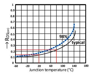
**Figure 6.** Variation of the  $R_{DS_{ON}}$  with respect to temperature variation.
