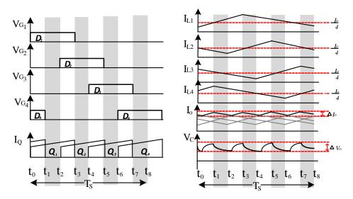
Figure 4. Waveforms during a commutation period.
