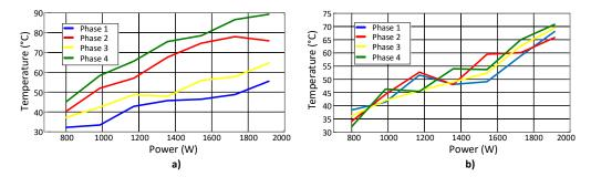
Figure 14. Behavior of temperature in switches (a) imbalanced currents, (b) balanced currents.
