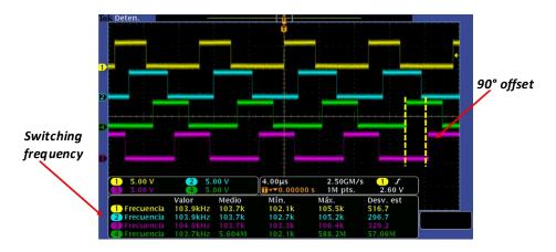
Figure 9. Commutation signals for phases with the corresponding 90° phase shift and duty cycle (40%).
