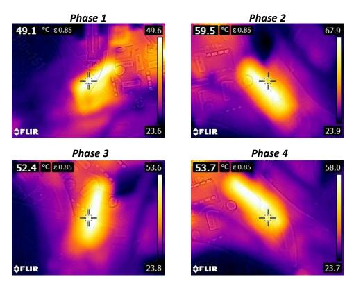
Figure 13. Temperature spectrum with balanced phases of the converter.
