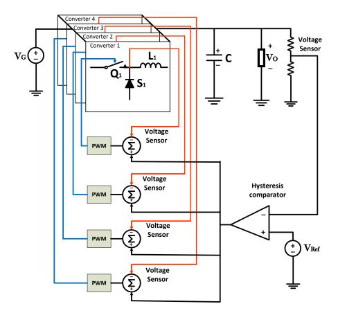
Figure 5. General control diagram for current balance by a phase based on [43].
