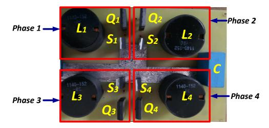
Figure 8. Functional prototype of the MBC.
