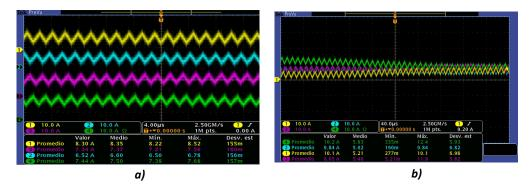
**Figure 11.** Current signals with the current balance scheme (**a**) balanced currents, (**b**) operation of the current balance scheme ( $\approx 240 \,\mu S$  stabilization response).
