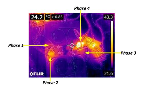
Figure 12. Temperature spectrum with imbalanced phases of the converter.
