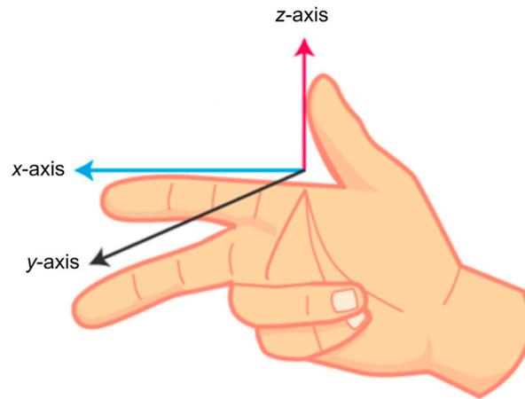
**Figure 8.** Right-handed coordinate system.
