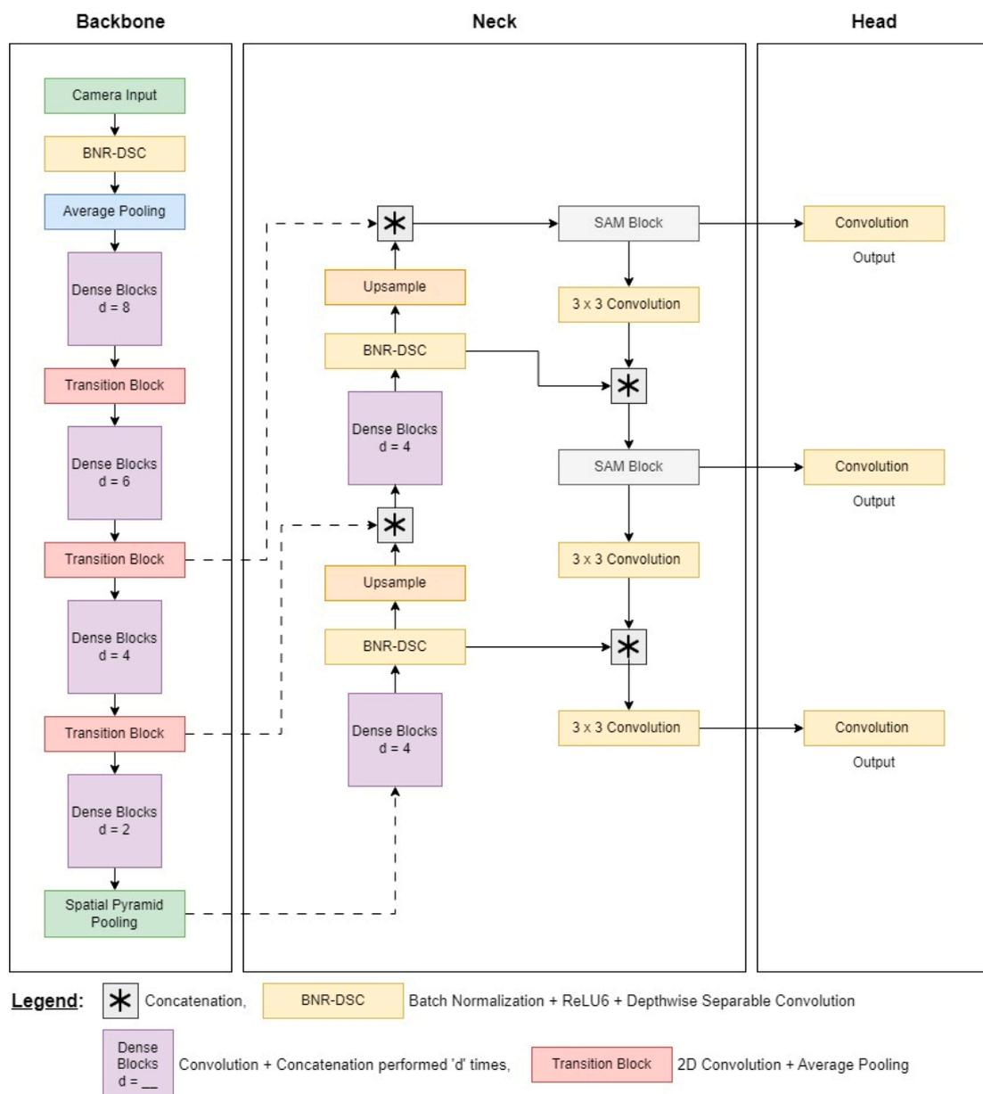
Figure 3. NextDet architecture utilized as the baseline for the proposed NeXtFusion architecture.
