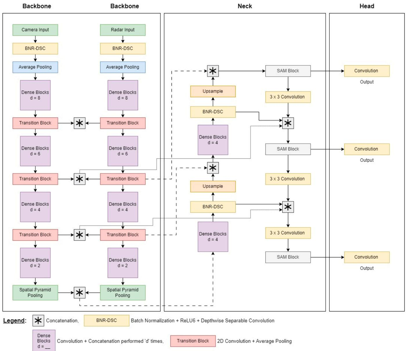
Figure 9. Architecture of the proposed NeXtFusion 3D object detection network.
