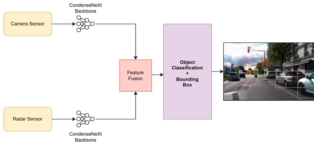
**Figure 1.** An overview of the proposed NeXtFusion multi-modal sensor fusion neural network.
