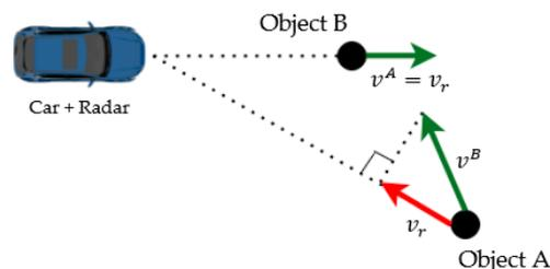
**Figure 2.** Comparison between velocities: the true velocity ( $v^A$ ) for object A is equal to the radial velocity ( $v_r$ ), whereas, for object B, the radar-reported radial velocity ( $v_r$ ) indicated by the red arrow is not equal to the true velocity ( $v^B$ ).
