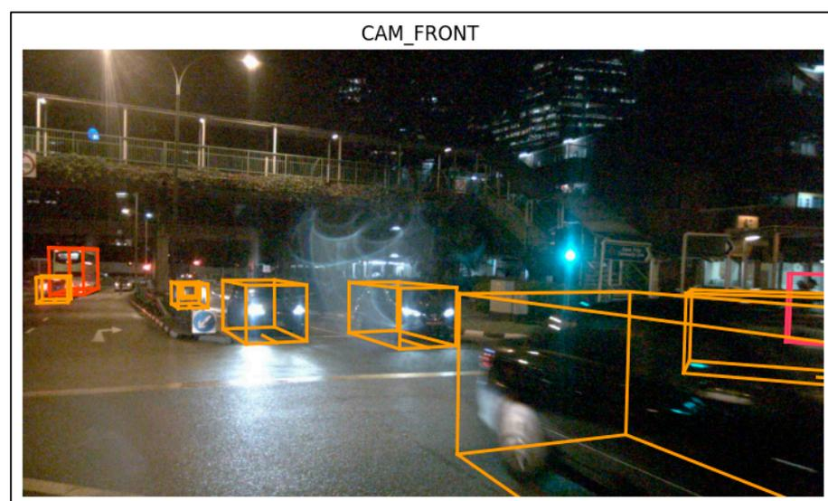
**Figure 11.** An example of Camera-Radar fusion-based 3D object detection involving occlusion at night from the nuScenes dataset using the proposed NeXtFusion network. Different colors of the bounding boxes indicate different objects detected.
