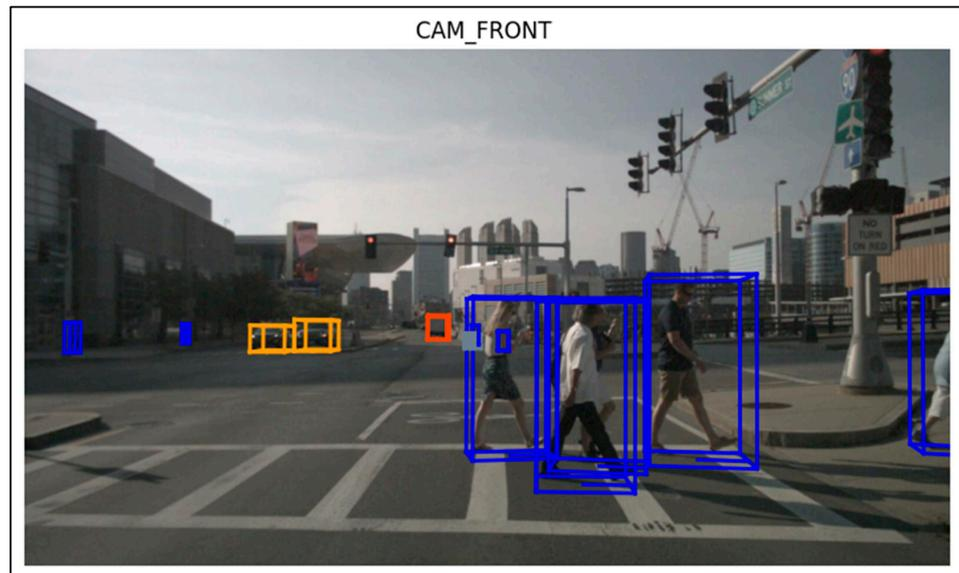
**Figure 12.** An example of Camera-Radar fusion-based 3D object detection at an intersection using the proposed NeXtFusion network. Here, blue bounding boxes, denote people, yellow bounding boxes denote cars and red bounding boxes denote bus.
