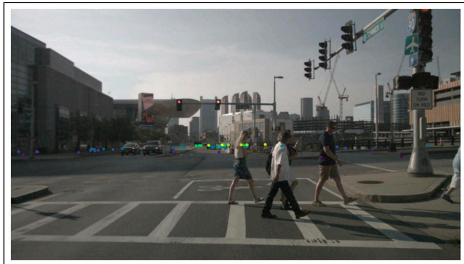
**Figure 13.** An illustration of radar point-cloud data of the environment from the nuScenes dataset generated by NeXtFusion. Dots represent objects, with darker shades indicating closer proximity to the sensor.
