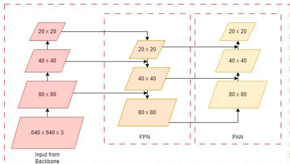
**Figure 4.** A visual depiction of top-down and bottom-up implementation of FPN and PAN networks.
