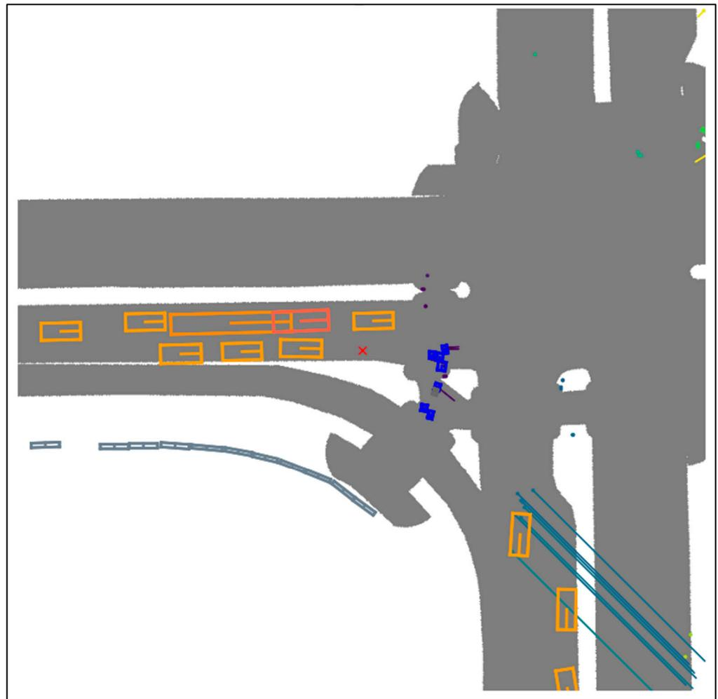
**Figure 14.** An example of very confident radar returns from two vehicles, captured and combined using five radar sweeps. Light blue lines indicate radar detection, indicating its length and orientation. Red cross indicates vehicle's ego-centric position. Here, blue bounding boxes, denote people, yellow bounding boxes denote cars and red bounding boxes denote bus.
