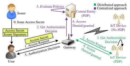
**Figure 20.** Access-control approach. Policy Decision Point (PDP) is a service that makes authorization decisions. PDP is either offered by an external entity or embedded into an IoT device.
