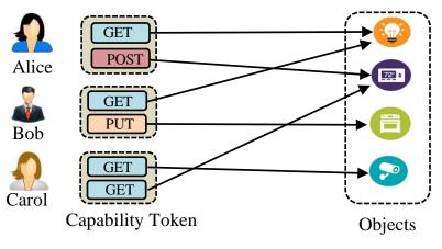
(**b**) CapBAC model. **Figure 19.** RBAC vs. CapBAC model.
