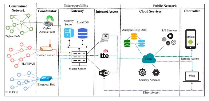
Figure 3. The operational model of an IoT system.
