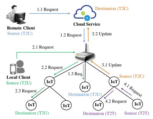
Figure 4. Communication interfaces in an IoT system.
