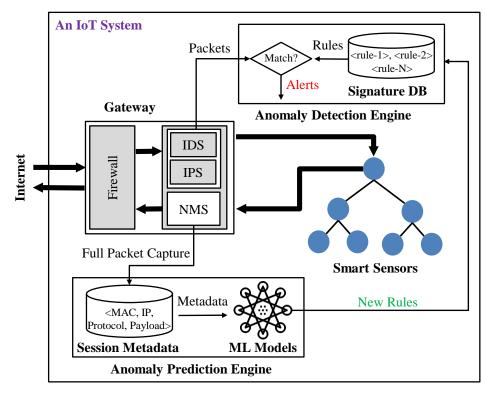
**Figure 28.** An adaptive anomaly-detection system. NMS = Network Monitoring System. ML = Machine Learning.
