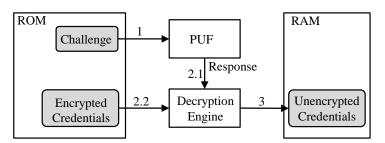
Figure 27. A PUF-based scheme for storing credentials securely.
