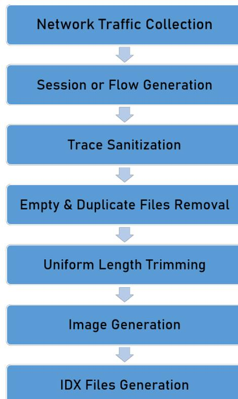
**Figure 2.** The detailed process of data preprocessing.
