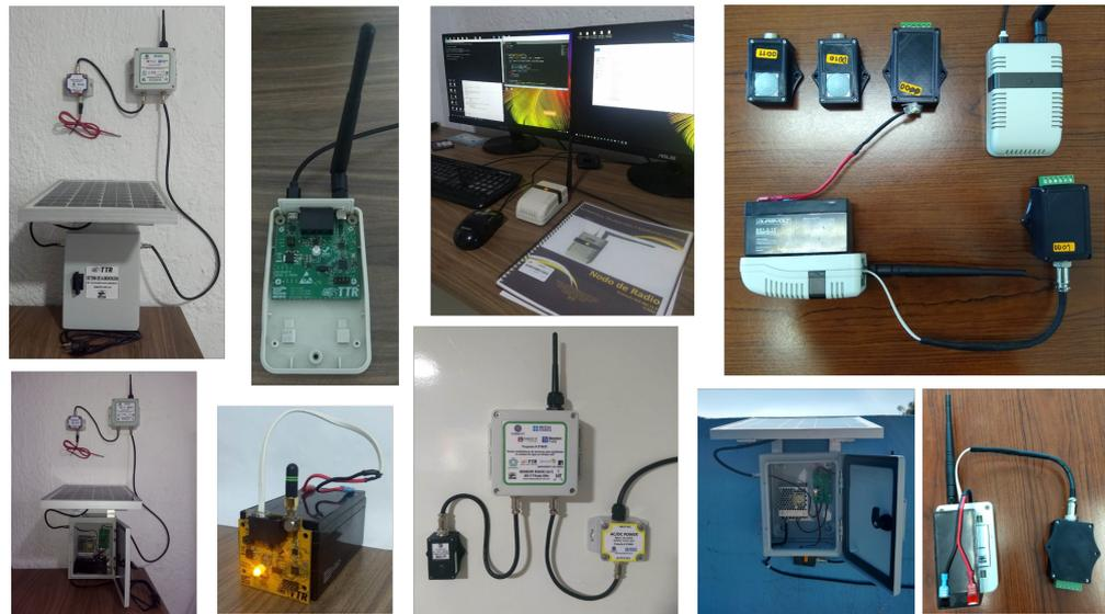
**Figure 1.** Real implementation of the sensor network.
