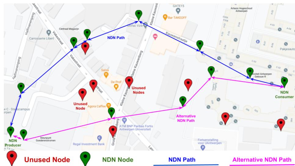
Figure 1. Example of NDN communication over CityLab testbed [4].
