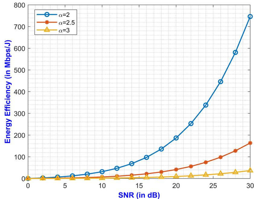
**Figure 3.** EE vs. threshold SNR for varying path loss exponents.
