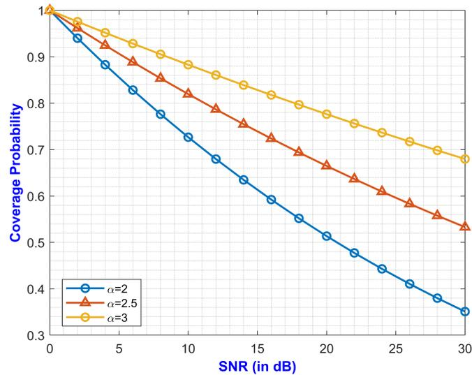
Figure 4. Coverage probability vs. threshold SNR for varying path loss exponents.
