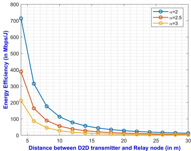
Figure 5. EE vs. distance between the D2D transmitter and the relay node for varying path loss exponents.
