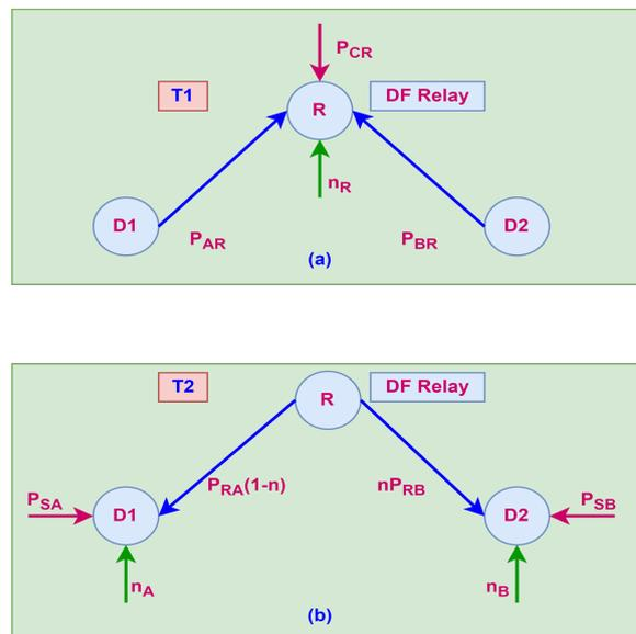
**Figure 2.** Line diagram representing the bidirectional exchange of information between  $D_1$  and  $D_2$  through the DF relay in the presence of interference and noise in different time slots. (a) time slot  $T_1$  and (b) time slot  $T_2$ .
