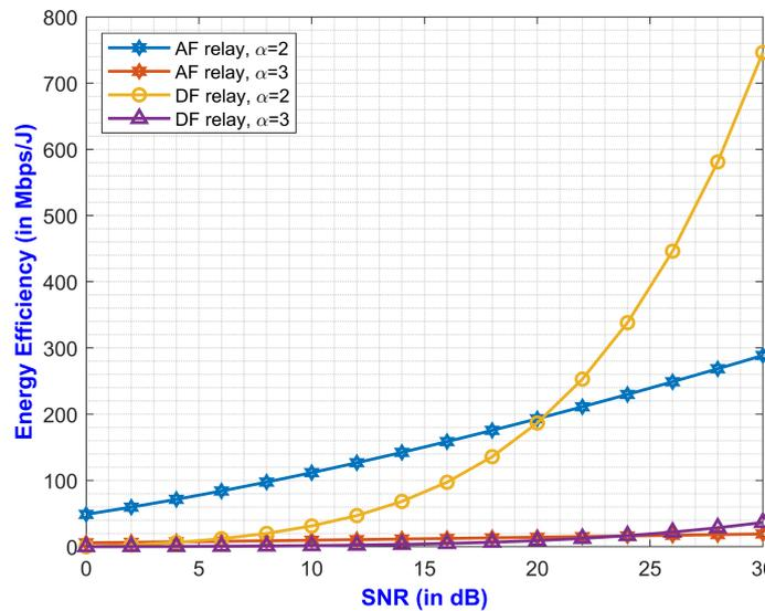
Figure 6. Comparison of the EE for the DF and AF relay schemes.
