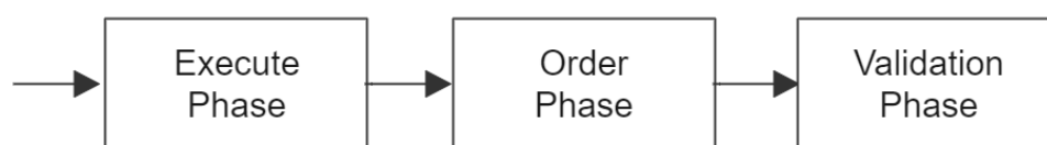
Figure 6. Execute-order-validate transaction processing model.
