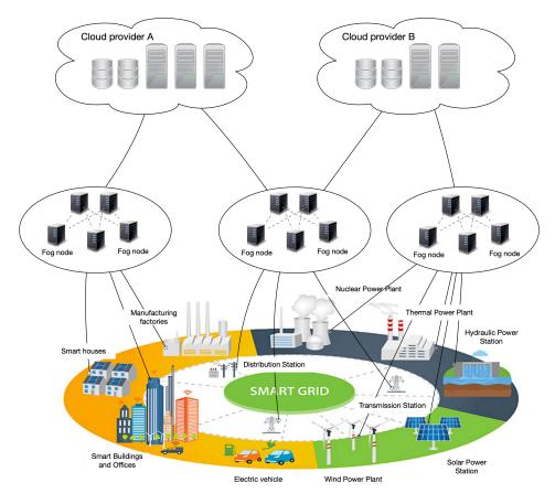
Figure 6. A fog-cloud-based architecture for smart grids.
