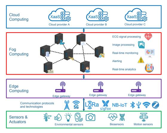
Figure 5. Fog-cloud-based architecture for healthcare.
