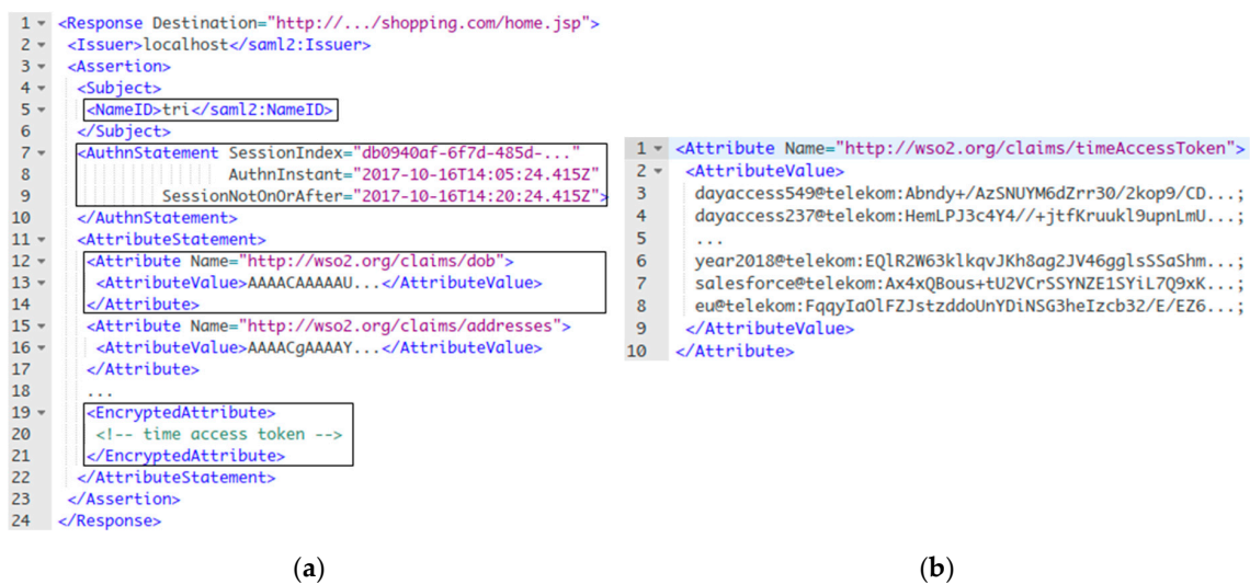
Figure 15. (a) SAML response with encrypted time access token; (b) Time access token.
