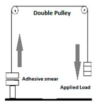
Figure 1. Illustration of determination of binding strength by double pulley apparatus.
