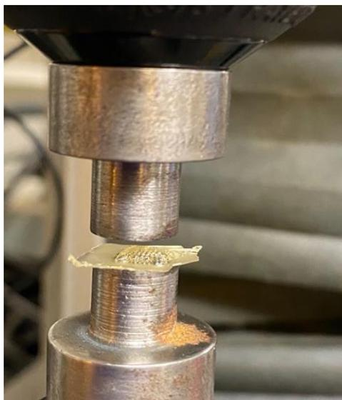
**Figure 3.** Mechanical station for fracture test under axial force.
