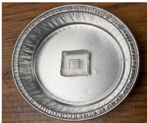
**Figure 2.** PDMS female microneedle array mold.
