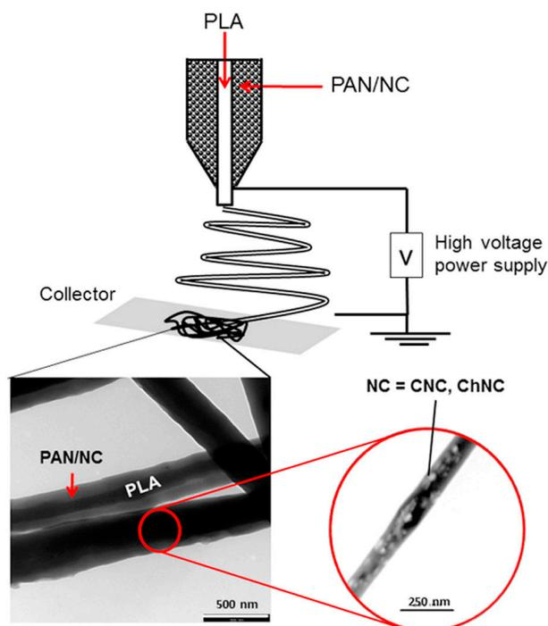
**Figure 6.** Transmission electron microscopy pictures of core–shell nanofibers prepared by coaxial Electrospinning technology. Published by Elsevier, 2022 [140].
