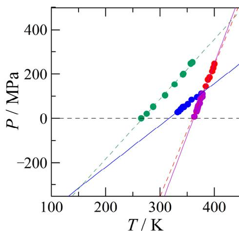
**Figure 8.** The pressure–temperature phase diagram based exclusively on the obtained HP-DTA data measured in the current study (equilibrium I–II dark blue, equilibrium II–L purple, equilibrium I–L red) and previously measured data (equilibrium III–II green) [1].
