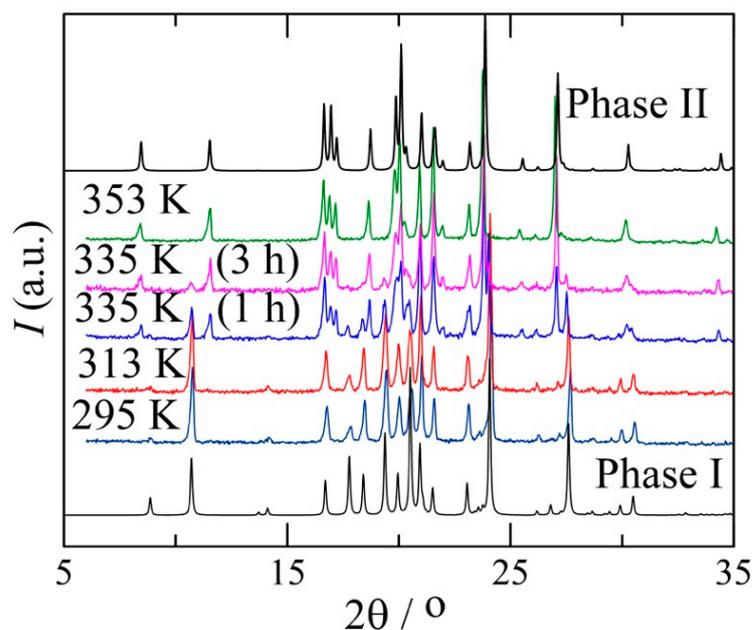
**Figure 3.** Benzocaine form I at 295 K (22 °C) after recrystallisation in ethanol. At 313 K (40 °C), form I still appears to be stable; however, further heating slowly leads to the formation of form II starting at 335 K (62 °C), as demonstrated by two measurements, 1 h each, at this temperature. Form II is clearly the only polymorph present at 353 K (80 °C). The diffraction patterns of phases I and II (in black) have been provided based on single-crystal diffraction data from the CSD.
