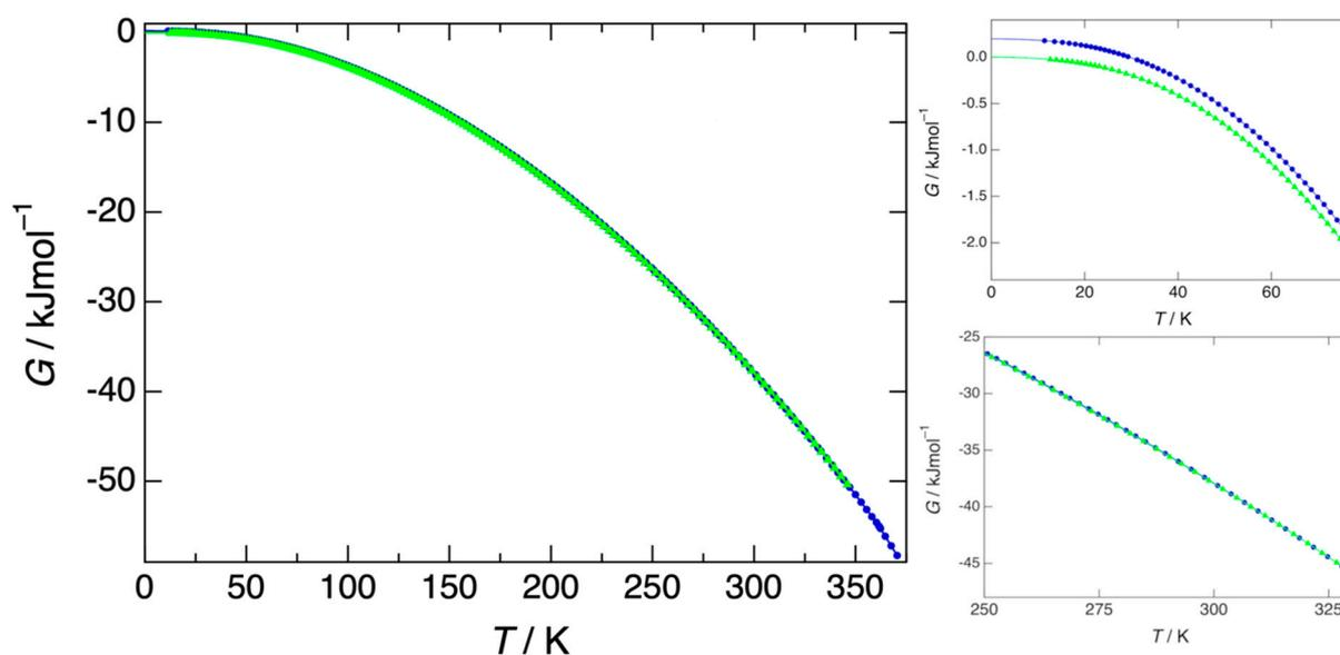
**Figure 7.** Gibbs free energy of form I (green triangles) and form III (blue circles), which become equal once both forms have turned into form II (bottom right-hand figure). Form III has a higher Gibbs free energy (top right-hand figure), and is therefore less stable than form I. Form I remains the most stable form to 319.5 K.
