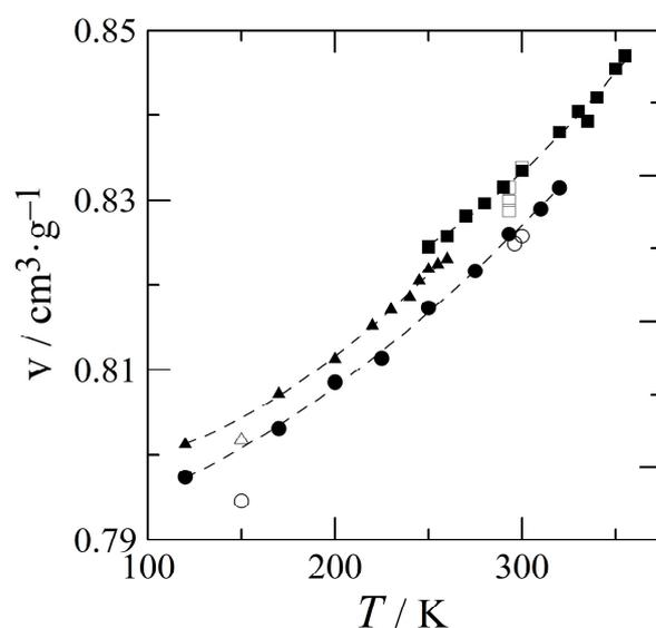
**Figure 4.** Specific volumes of forms I (filled circles), II (filled squares), and III (filled triangles) obtained by powder X-ray diffraction in the current study. Single-crystal literature data are indicated by open symbols.
