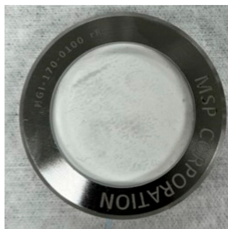
Figure 11. Filter cassette to keep the glass fiber filter and the pre-soaked polycarbonate filter.
