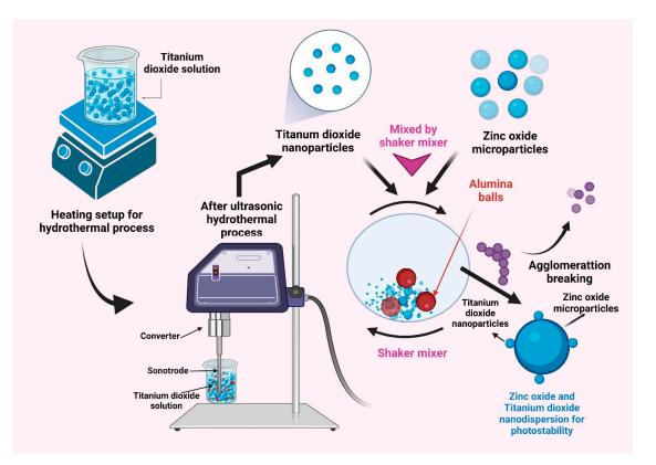
**Figure 7.** The nanodispersion of titanium dioxide nanoparticles and zinc oxide microparticles is achieved with a shaker mixer by using an alumina ball. Prior to mixing, titanium dioxide nanoparticles were prepared by using hydrothermal and ultrasonic treatment. The shaker mixer ensures agglomeration breaking and provides photostable nanodispersions ready for drug use.
