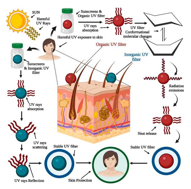
**Figure 8.** The interaction of organic and inorganic UV filters from sunscreen formulation with UV light. The organic UV filter undergoes conformational changes after UV exposure, followed by heat release. The organic UV filter works through the reflection, scattering or absorption of UV light.
