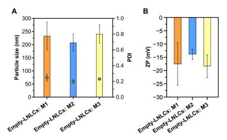
**Figure 2.** Physicochemical properties of empty LNLCs prepared by hydrotrope method (M1), lipid film hydration method (M2) and emulsification method (M3): (**A**) size and polydispersity index (PDI), and (**B**) surface charge (zeta potential, ZP). The data are expressed as mean  $\pm$  standard deviation of three independent measurements.
