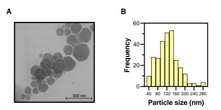
Figure 6. (A) STEM photograph of empty LNLCs M3 at 200 kV  $\times$  80.00 k. (B) Size distribution histogram of empty LNLCs M3.
