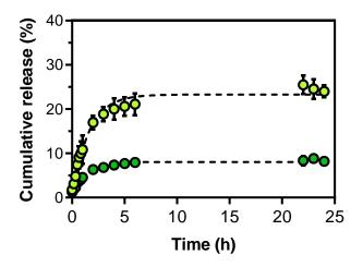
**Figure 9.** Cumulative DOX release profile from the LNLCs M3 at pH 5.5 (stimulated endosomal environment) (light green data) and pH 7.5 (stimulated physiological/plasma environment) (dark green data) as a function of time (25 h). The data are expressed as mean  $\pm$  standard deviation of three independent measurements. The lines represent the best kinetic fit obtained according to the first-order model.
