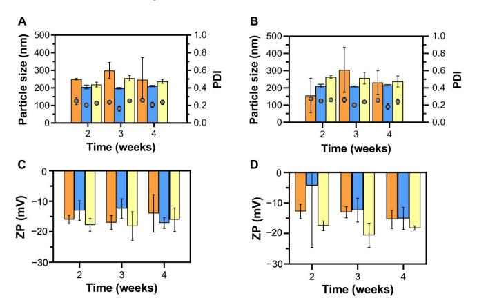
**Figure 3.** Stability of empty LNLCs prepared by hydrotrope method (M1, orange data), lipid film hydration method (M2, blue data) and emulsification method (M3, yellow data) during 4 weeks in different storage conditions: (**A**) size and PDI at 25 °C, (**B**) size and PDI at 4 °C, (**C**) surface charge (ZP) at 25 °C, and (**D**) surface charge (ZP) at 4 °C. The data are expressed as mean  $\pm$  standard deviation of least three independent experiments.
