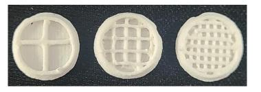
Figure 2. The section of F4–F6 with different infill percentages, 10%, 30%, and 50% from left to right.
