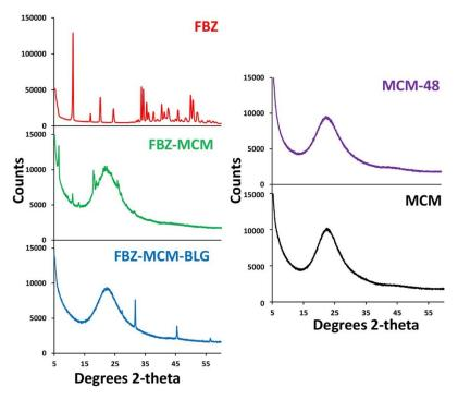
Figure 3. XRD pattern of the synthesized MCM-48, MCM, FBZ-MCM, and FBZ-MCM-BLG nanoparticles.
