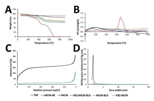
**Figure 2.** (**A**) TGA thermogram of FBZ, MCM-48, MCM, FBZ-MCM, MCM-BLG, and FBZ-MCM-BLG nanoparticles; (**B**) DSC thermogram of FBZ, MCM-48, MCM, FBZ-MCM, MCM-BLG, and FBZ-MCM-BLG nanoparticles; (**C**) N2 adsorption-desorption isotherms; and (**D**) pore size distributions of MCM and FBZ-MCM nanoparticles using the BET method.
