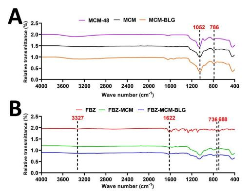
**Figure 4.** Fourier transform infrared spectroscopy (FTIR) spectra of (**A**) MCM-48, MCM, and MCM-BLG; and (**B**) FBZ, FBZ-MCM, and FBZ-MCM-BLG nanoparticles. The peaks at 1622, 736, and 688 cm<sup>-1</sup> regions in the spectra of FBZ, FBZ-MCM, and FBZ-MCM-BLG nanoparticles prove that (i) FBZ was loaded into these nanoparticles and (ii) the chemical structure of the drug remained intact, meaning that FBZ was physically loaded into these NPs.
