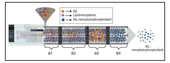
**Figure 1.** An illustration of TSP to obtain SIL-nanophytophospholipid. B1, B2, B3 and B4 represent the barrel heating zone.
