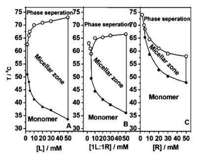
**Figure 3.** Comparative phase behavior of a normal Pluronic (L44), a reverse Pluronic (10R5) and a 1:1 mixture of both. Reproduced with permission from [15], Copyright American Chemical Society 2012.
