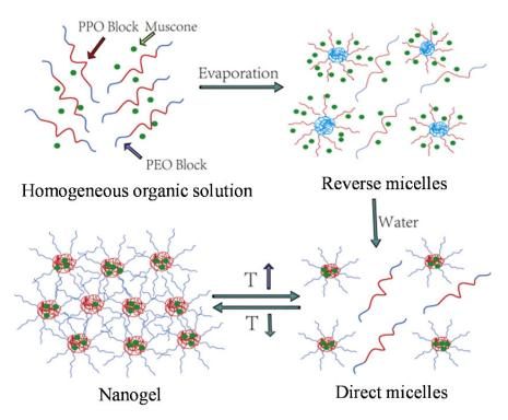
**Figure 6.** Design of muscone thermoresponsive nanogels prepared by  $\text{RM} \rightarrow \text{PM}$  method. Reprinted from [118], Copyright 2017, with permission from Elsevier.
