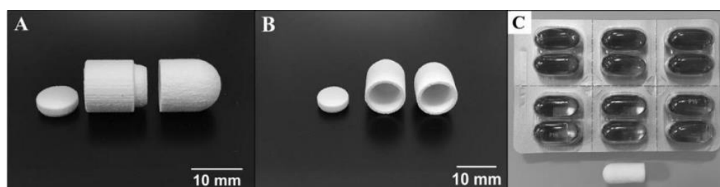
Figure 11. Multi-compartment preform tablet. (A) Side view of the three pieces constituting the preform tablet. From left to right, top cap, top compartment, and bottom compartment. These pieces were manufactured by powder-bed 3D printing using binder DI water with 5% ethanol and 0.25% Tween 80. The powder utilized for their construction was calcium sulfate. Each of the two wells has a 250 \mu\text{L} capacity. (B) Front view of the preform tablet fabricated. (C) Comparison between the assembled version of the preform tablet and commercially available gel capsules [74].
