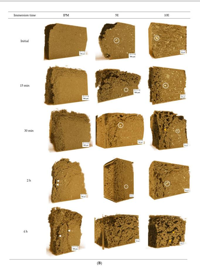
**Figure 7.** (**A**) Surface and (**B**) cross-sectional reconstructed 3D images of IBU-P407 effervescent matrix tablets in pH-changed media at various immersion times.
