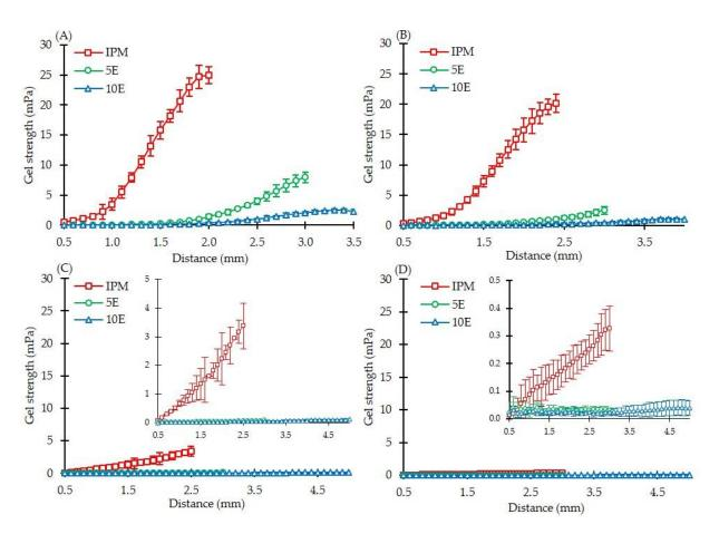
**Figure 4.** Gel strength profiles of IBU-P407 effervescent matrix tablets at different immersion times (n = 5); (**A**) 15 and (**B**) 30 min; (**C**) 2 and (**D**) 4 h.
