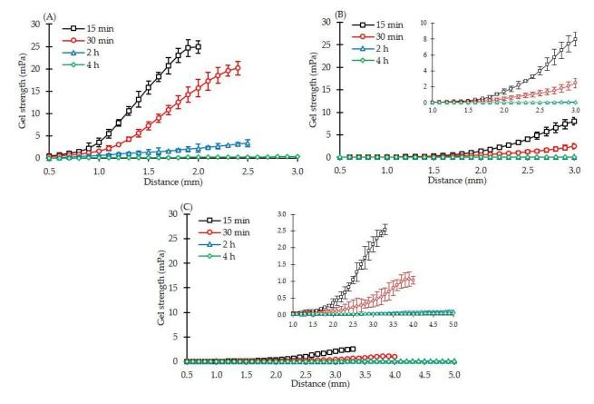
**Figure 3.** Gel strength profiles of IBU-P407 effervescent matrix tablets (n = 5); (**A**) IPM, (**B**) 5E and (**C**) 10E.
