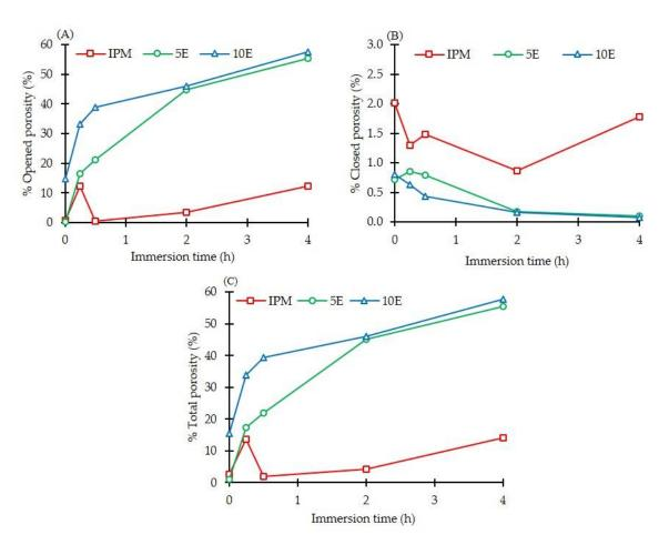
**Figure 8.** (**A**) Opened, (**B**) closed and (**C**) total porosities of IBU-P407 effervescent matrix tablets in pH-changed media at various immersion times.
