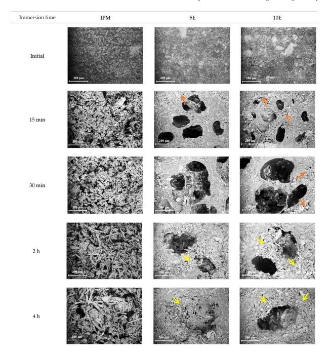
**Figure 6.** SEM micrographs of IBU-P407 effervescent matrix tablets in pH-changed media at various immersion times (magnification: 250×).
