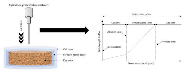
Figure 1. Schematic representation of gel strength determination upon hydration.
