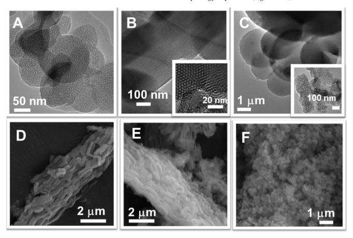
**Figure 4.** TEM images of MCM-48C (**A**), SBA-15 (**B**) and MCF (**C**) and SEM micrographs of SBA-15 (**D**), SBA-15-SH (**E**) and SBA-16 (**F**) carriers.
