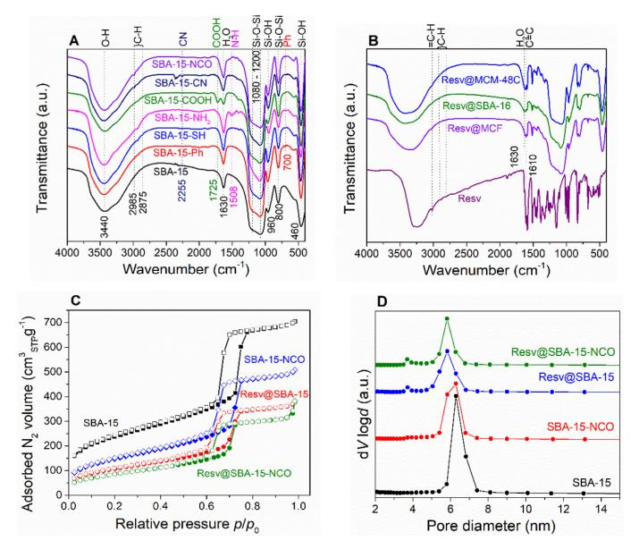
**Figure 1.** FT-IR spectra of pristine and functionalized SBA-15 (**A**) and resveratrol–loaded pristine silica carriers (**B**); representative nitrogen adsorption-desorption isotherms of pristine and functionalized SBA-15 carriers and corresponding resveratrol-loaded carriers (**C**) and pore size distribution curves of the same selected SBA-15-type carriers and resveratrol-loaded materials (**D**).
