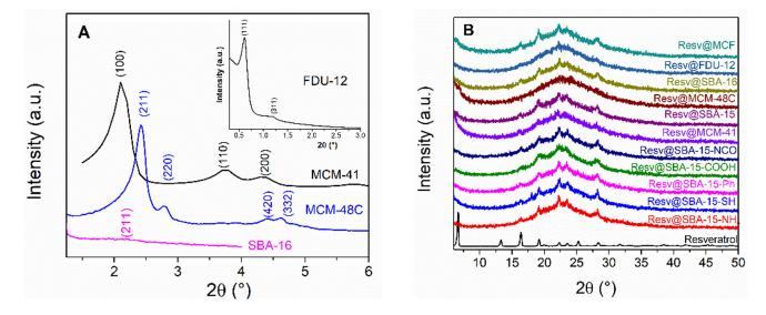
**Figure 2.** Small–angle XRD patterns of mesoporous silica carriers (**A**) and wide-angle XRD patterns of resveratrol loaded carriers (**B**).
