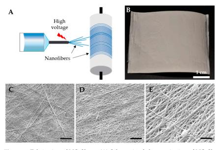
**Figure 1.** Fabrication of NO-fibers. **(A)** Schematic of electrospinning of NO-fibers. The polymer solution is emitted through the needle when high voltage is applied to the tip of the needle and fibers are collected on a rotating collector; **(B)** photograph of an electrospun sheet of PVP NO-fibers. Scanning electron microscope images of PVP NO-fibers: **(C)** PROLI–NO-fibers; **(D)** DPTA–NO-fibers; **(E)** DETA–NO-fibers. Scale bar: 5 μm.
