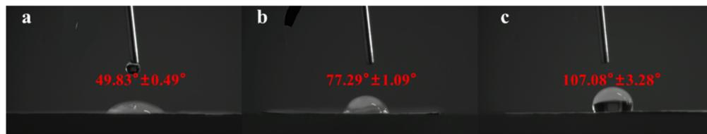
**Figure 4.** The contact angle (CA) measurement of ART-loaded PCL/Col nanofibers with different polymer ratios: (a) PCL/Col-A; (b) PCL/Col-B; (c) PCL/Col-C.
