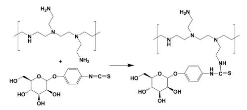
**Figure 2.** Reaction scheme for the synthesis of Man-PEI. PEI1800 reacted with  $\alpha$ -D-Mannopyranosylphenyl isothiocyanate for 24 h to produce Mannosylated PEI. The product was purified through dialysis.
