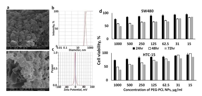
**Figure 7.** PEG-PCL NPs with encapsulated Man-PEI/plasmid complexes present nanosized spherical structures of relatively similar size and minimal toxicity. (a) Representative SEM imaging of the polymer nanocarriers; (b) Dynamic Light Scattering analysis of the nanoparticles; (c) Zeta-potential analysis of the nanocarriers; (d) Cytotoxicity analysis of PEG-PCL NPs with encapsulated Man-PEI/plasmid complexes in SW480 and HCT-15 cells.
