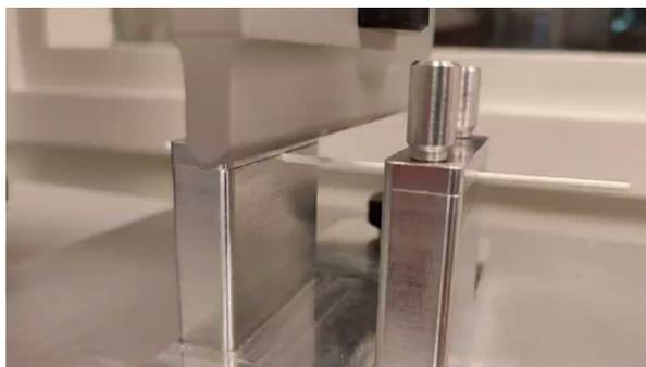
**Figure 1.** 3 points bending setup with attached filament.
