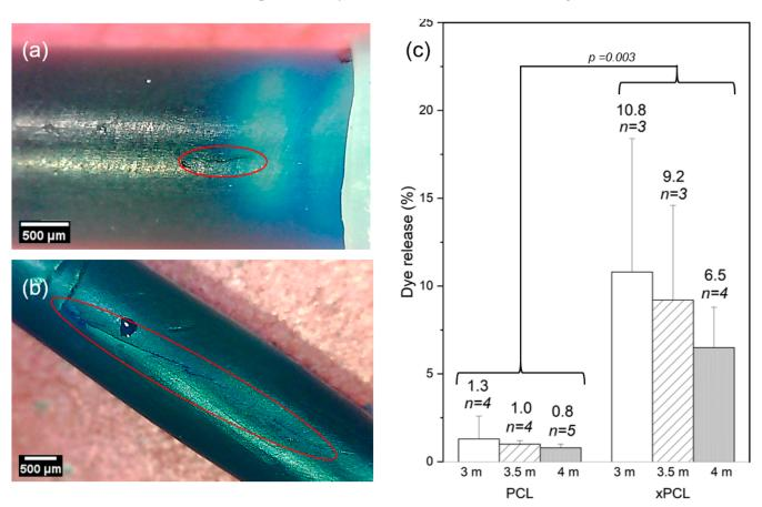
**Figure 4.** Moment of burst. Microscope images of representative burst sites of a PCL tube (**a**) and a xPCL tube (**b**). Red ovals are to highlight the lengths of the burst areas. Fissure lengths circa 0.7 mm (**a**), and 5 mm (**b**). (**c**) Average percentage of loaded dye released upon burst of the devices. Error bars represent standard deviation. Population sizes are indicated above each bar along with the %-age of dye released.
