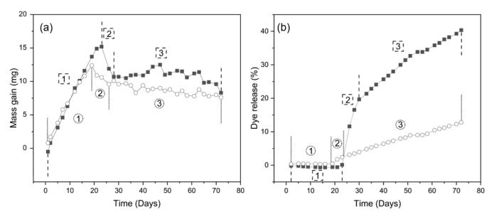
**Figure 2.** Phases of osmosis-driven delayed burst release, demonstrated through mass change (a) and dye release (b) profiles of one representative capsule each of PCL ( $\bigcirc$ ) and xPCL ( $\blacksquare$ ) 3.5 m devices. Phases are shown as (1) water uptake, (2) post-burst stabilisation, and (3) steady-state release. The point of burst is depicted by the dashed lines that separate phases 1 and 2.
