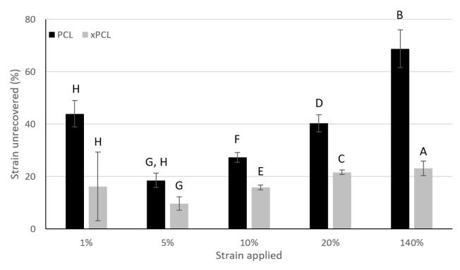
**Figure 1.** Comparison of the average permanent set following each target strain exerted. Data are normalised against the strain applied. Recovery time after each strain was 15 min. Error bars indicate standard deviation. Groups that do not share a letter are statistically different from one another (p < 0.05). PCL p = 1, xPCL p = 1.
