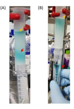
**Figure S1.** SEC method for removing free dyes. (A) SEC column before collecting exosomes. (B) SEC Column after collecting exosomes.
