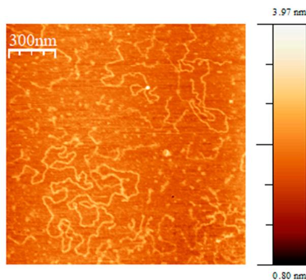
**Figure S9.** AFM topography image of DNA in extended-coil conformation adsorbed on APTES modified mica surface in cacodylate buffer (ionic strength = 1.63 mM, pH = 7.4),  $C_{DNA} = 0.3 \mu\text{M}$ .
