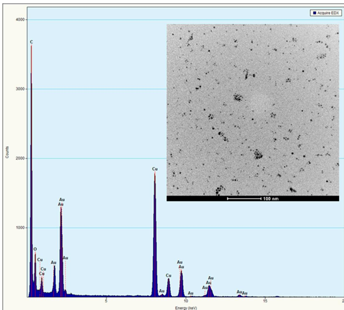
**Figure S7.** EDS spectrum of Au@16-Ph-16 nanoparticles. Elemental mapping results indicate the distribution of Gold element on the particles. Bear in mind that the presence of copper ion is due to the use of copper grid coated with a carbon film needed for TEM measurement.
