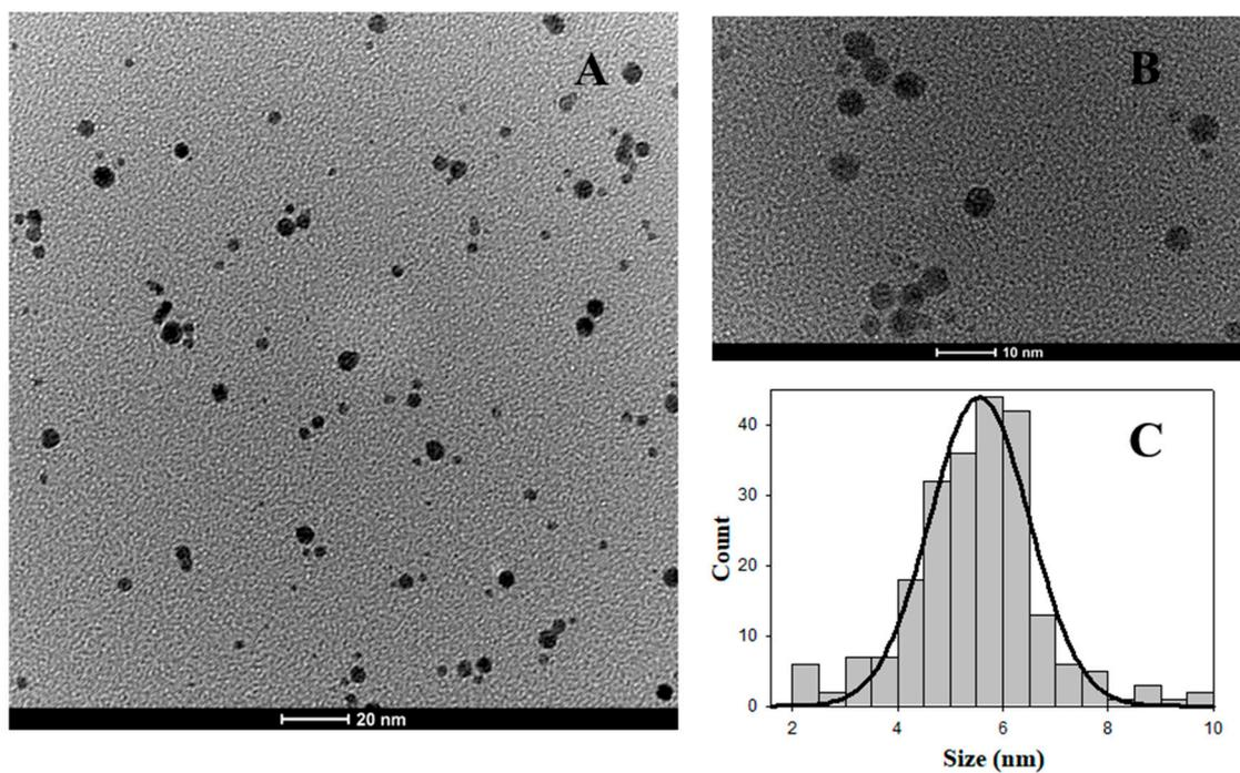
**Figure S6.** (A,B) TEM image of free Au@16-Ph-16 gold nanoparticles. (C) Size distribution of Au@16-Ph-16 in water.
