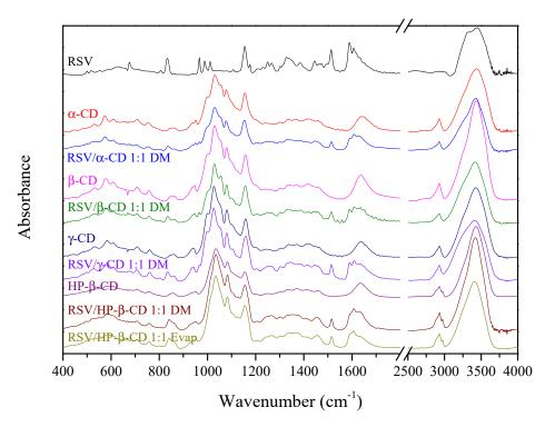
Figure 2. FT-IR spectra of selected powder resveratrol (RSV)/cyclodextrin (CD) systems.
