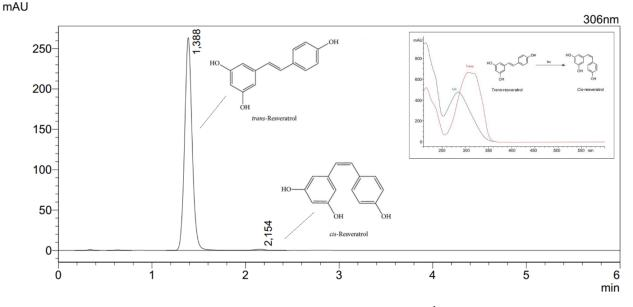
**Figure 3.** Chromatogram of RSV (c = 40  $\mu$ g mL<sup>-1</sup>).
