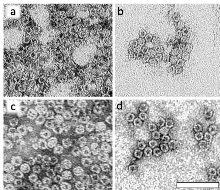
**Figure S2.** TEM representative images of native HFn (a), and after purification with Endotrap HD resins (b), Triton X-114 (c) and the combined method of the two (d). Scale bar = 50 nm.
