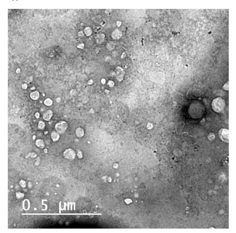
**Figure 1.** Transmission electron micrograph of the prepared liposomes P-lip (F4) when stained with uranyl acetate (2.5% w/v) with scale 0.5  $\mu$ m.
