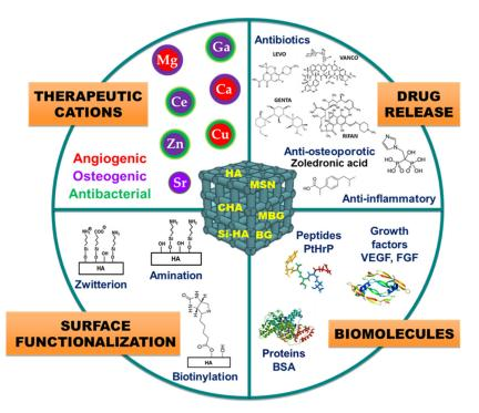
Figure 3. Representation of bioceramic scaffold modifications for bone regeneration.
