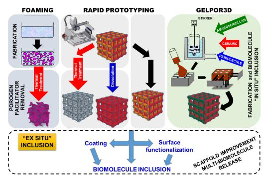
**Figure 1.** Schematic representation of the different scaffolds fabrication technologies employed as well as the additional routes designed to improve and tailor their final performance.
