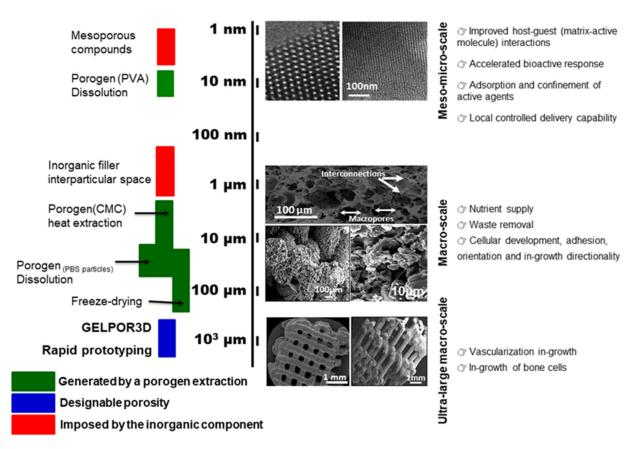
**Figure 2.** Schematic representation, related to the length scale, of the scaffolds pore distribution, the methods employed to obtain it, micrographs at different magnifications and the different physiological phenomena taking place (SEM micrographs reproduced with permission from Shruti et al. [10], Acta Biomater.; published by Elsevier, 2013 and Heras et al. [47], Acta Biomater.; published by Elsevier, 2019).
