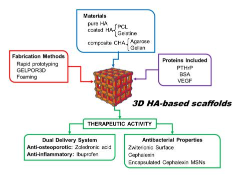
Figure 4. Strategies carried out in the fabrication of engineered HA-based scaffolds.
