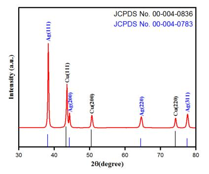
Figure 5. X-ray diffraction (XRD) pattern of Beta vulgaris assisted Ag-Cu bimetallic nanoparticles.
