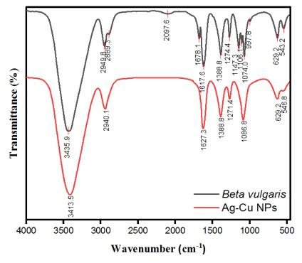
**Figure 4.** Fourier transforms infrared (FTIR) spectra of *Beta vulgaris* extract and Ag-Cu bimetallic nanoparticles.
