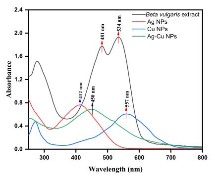
Figure 3. UV–Visible spectra of Beta vulgaris extract, Ag NPs, CuNPs and Ag-Cu bimetallic nanoparticles.
