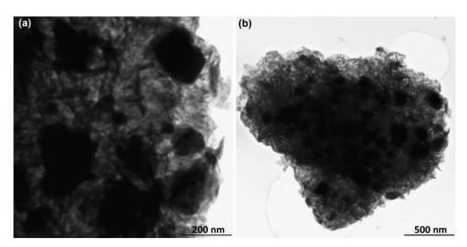
**Figure 7.** Transmission electron microscope (TEM) images of Ag-Cu bimetallic nanoparticles at different magnifications. (**a**) 200 nm and (**b**) 500 nm.
