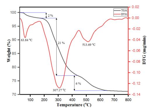
**Figure 8.** Thermogravimetric analysis (TGA) and derivative thermogravimetric (DTG) curves of Ag-Cu bimetallic nanoparticles.
