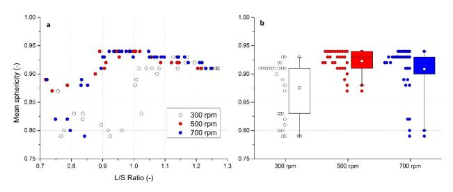
**Figure 6.** Evaluation of mean sphericity for impeller speeds of 300, 500 and 700 rpm: (**a**) effect of the L/S ratio on sphericity, (**b**) box charts of sphericity for different impeller speeds.
