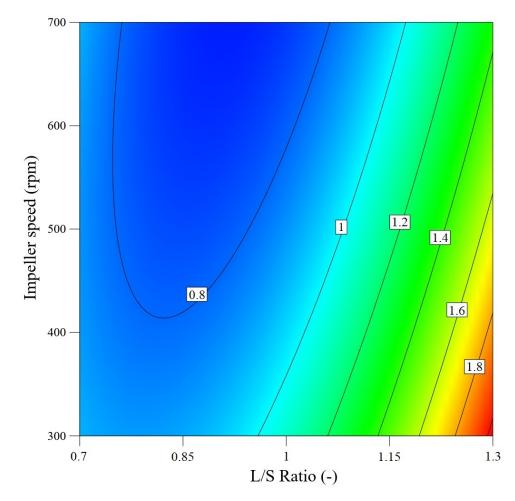
**Figure 13.** Contour plot of quadratic model for prediction of mean granule size as function of L/S ratio and impeller speed.
