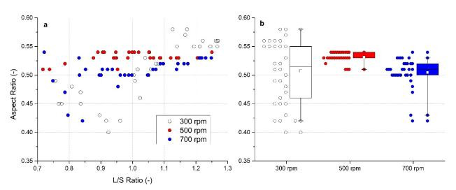
**Figure 7.** Evaluation of the aspect ratio for impeller speeds of 300, 500, and 700 rpm: (**a**) effect of the L/S ratio on aspect ratio, (**b**) box charts of aspect ratio for different impeller speeds.
