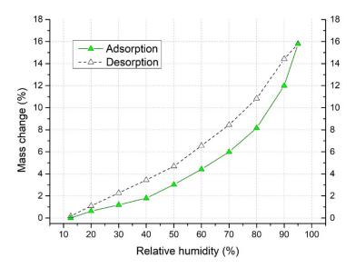
Figure 3. Adsorption and desorption isotherms of Avicel PH101 analyzed by Aquadyne DVS.
