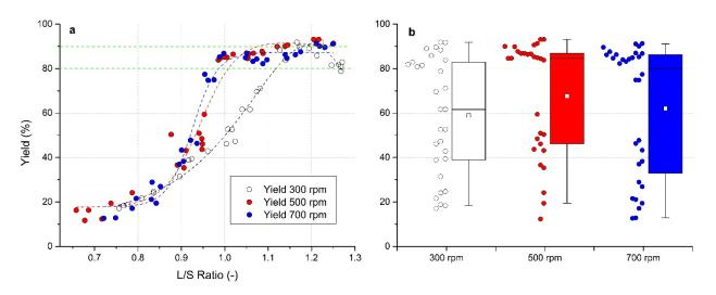
**Figure 5.** Evaluation of yield fraction (0.4–3 mm) for impeller speeds of 300, 500, and 700 rpm: (**a**) effect of the L/S ratio on yield fraction, green lines indicate yield interval from 80 to 90%, (**b**) box charts of yield fraction for different impeller speeds.
