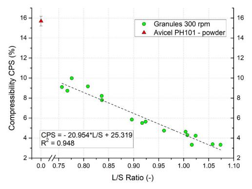
**Figure 12.** Compressibility of raw Avicel PH101 powder and effect of L/S ratio on compressibility of granules manufactured at 300 rpm impeller speed.
