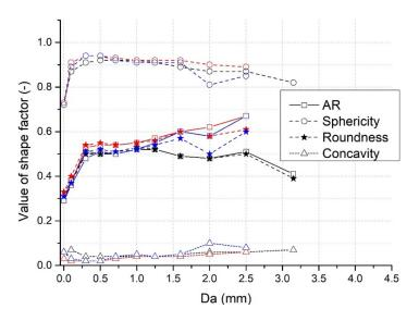
**Figure 10.** Relationship of investigated shape factors on area equivalent diameter  $D_a$  at the L/S ratio = 1.0 at impeller speeds of 300 (black), 500 (red), and 700 rpm (blue).
