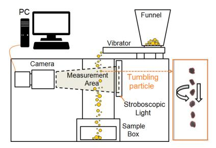
Figure 1. Principle of measurement by Dynamic image analysis (DIA) using PartAn 3D.
