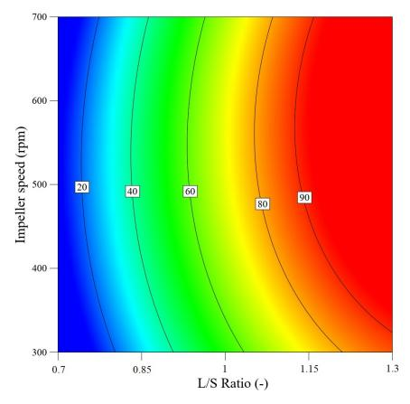
**Figure 14.** Contour plot of the quadratic model for prediction of the process yield as a function of L/S ratio and impeller speed.
