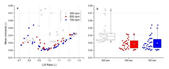
powder materials and granules [66]. Based on the results, the smoothest granules were formed at higher impeller speeds in the L/S range of 0.9 to 1.05.
