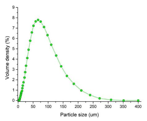
Figure 2. Particle size distribution of Avicel PH101 analyzed by Mastersizer 3000.
