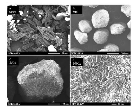
**Figure 11.** SED images of granules from electron microscope: (**a**) raw particles of Avicel PH101 at  $500 \times$  magnification, (**b**) granules produced at L/S  $\approx$  1.0 and 700 rpm impeller speed at  $50 \times$  magnification, (**c**) surface of granule at  $250 \times$  magnification, (**d**) detail of granule surface at  $1000 \times$  magnification.
