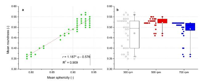
**Figure 8.** Evaluation of mean roundness. (a) Mean roundness relationship on mean sphericity, (b) box charts of mean roundness for impeller speeds 300, 500, and 700 rpm.
