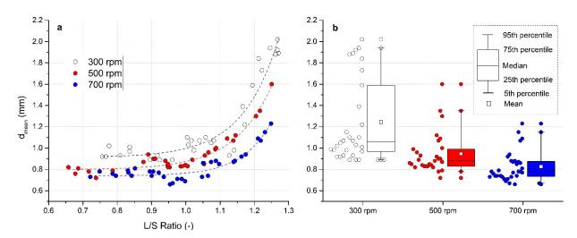
**Figure 4.** Evaluation of mean granule size for impeller speeds 300, 500, and 700 rpm: (**a**) effect of the L/S ratio on mean size  $d_{\text{mean}}$ , (**b**) box charts of  $d_{\text{mean}}$  for different impeller speeds. The picture shows a description of box charts.
