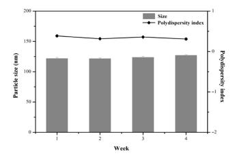
**Figure 6.** Particle size and size distribution of MPT0B291-human serum albumin (HSA) nanoparticles (NPs) stored at 4 °C for 4 weeks after reconstitution. Each point represents the mean  $\pm$  SD. Error bars represent the standard deviation (*n* = 3).
