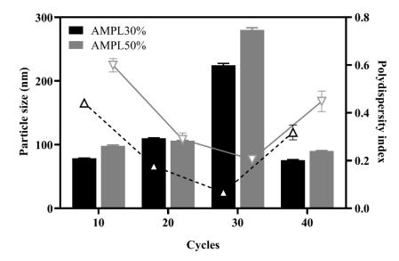
**Figure 2.** Effects of different amplitudes (AMPLs) of ultrasonication and different cycles of highpressure homogenization on the particle size and size distribution. Column: particle size (nm); line: polydispersity index. Each point represents the mean  $\pm$  SD. Error bars represent the standard deviation (n = 3).
