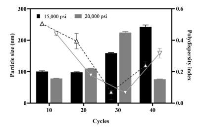
**Figure 3.** Effects of different pressures of high-pressure homogenization at different cycles on the particle size and size distribution. Column: particle size (nm); line: polydispersity index. Each point represents the mean  $\pm$  SD. Error bars represent the standard deviation (n = 3).
