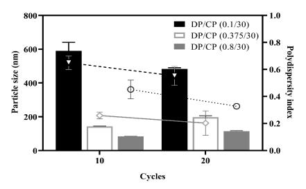
**Figure 4.** Effects of different ratios of the dispersed phase (DP) and continuous phase (CP) and different cycles of high-pressure homogenization on the particle size and size distribution. Column: particle size (nm); line: polydispersity index. Each point represents the mean  $\pm$  SD. Error bars represent the standard deviation (n = 3).
