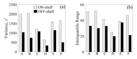
**Figure 8.** Variance (**a**) and Interquartile range (**b**) of the resulting pore size distribution for all VISF tests. In both bar plots, A, B and C are tests at 271 K while D, E and F are tests at 263 K. The solutions used are 5% sucrose (A,D), 5% mannitol (B,E) and 10% dextran (C,F).
