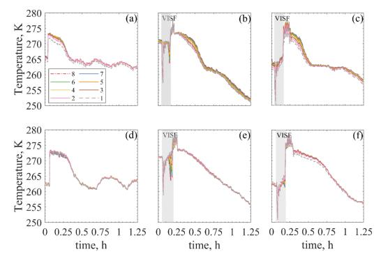
**Figure 4.** Axial temperature profiles during freezing of 5% sucrose. The top graphs (**a**–**c**) are ON-shelf, while bottom graphs (**d**–**f**) are OFF-shelf. (**a**,**d**) Spontaneous nucleation, (**b**,**e**) VISF 271 K, (**c**,**f**) VISF 263 K.
