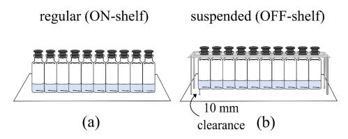
**Figure 1.** Experimental setup representations (not to scale): (**a**) the ON-shelf and (**b**) OFF-shelf vial configurations used.
