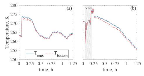
**Figure 6.**  $T_{max}$  and  $T_{bottom}$  during spontaneous nucleation (**a**) and VISF (**b**) at 271 K. (These are the same tests represented in Figure 4d,e.
