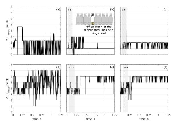
**Figure A4.** Range of measured  $H_{max}$  profile values for a single vial for sucrose 5%. Top graphs (**a**–**c**) are ON-shelf, while bottom graphs (**d**–**f**) are OFF-shelf. (**a**,**d**) Spontaneous nucleation, (**b**,**e**) VISF 271 K, (**c**,**f**) VISF 263 K.
