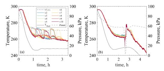
**Figure 3.**  $T_{bottom}$  freezing profiles of the spontaneous nucleation (**a**) and VISF at 263 K (**b**) in the case of OFF shelf vials and 5% sucrose.
