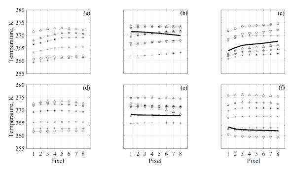
**Figure A3.** Vertical temperature gradients and possible profile inversions for sucrose 5%. Top graphs (**a**–**c**) are ON-shelf, while bottom graphs (**d**–**f**) are OFF-shelf. (**a**,**d**) Spontaneous nucleation, (**b**,**e**) VISF 271 K, (**c**,**f**) VISF 263 K. Each line represents the temperature gradient in the points of interest, represented by different symbols as shown in Figure A2.
