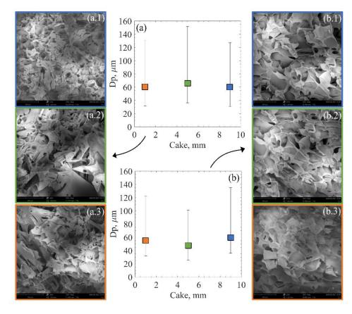
**Figure 7.** Average pore sizes for the resulting mannitol 5% cake after VISF tests at 271 K for ON-shelf (**a**) and OFF-shelf vials (**b**). The numbers after the test type letters (**a**,**b**) represent the cake section: (1) top, (2), middle and (3) bottom for the corresponding SEM images. The variability is expressed as the 3rd (**top**) and 1st (**bottom**) quartiles, as previously done for pore size data [28,35].
