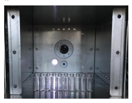
**Figure A1.** Picture of the box used with the IR sensor behind it and 10 vials placed ~25 cm from the sensor, as set for the experiments. The front wall of the box was removed for the picture.
