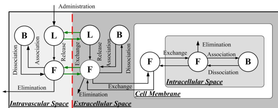
**Figure 2.** Drug transport in liposome-mediated delivery combined with FUS-MB-induced BBBD. The red dashed line refers to the disrupted BBB, and the enhanced transvascular transport is highlighted in green.
