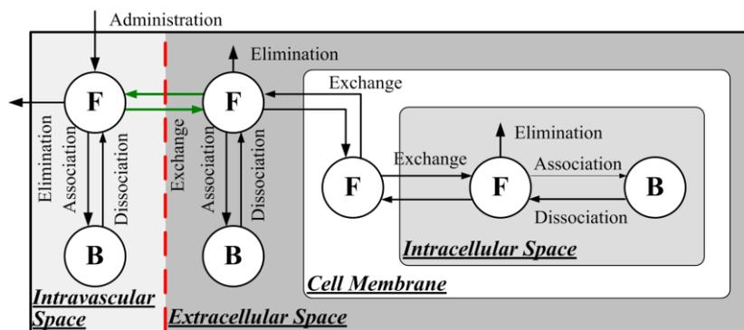
**Figure 1.** Transport processes involved in direct drug delivery in combination with focused-ultrasound-and-microbubble (FUS-MB)-induced blood–brain barrier disruption (BBBD). Red dashed line indicates the disrupted BBB, and the enhanced transvascular transport processes are highlighted in green.
