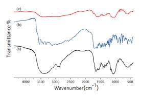
Figure S2. FT-IR spectra of (a) FA-conjugated CS, (b) FA, and (c) CS.
