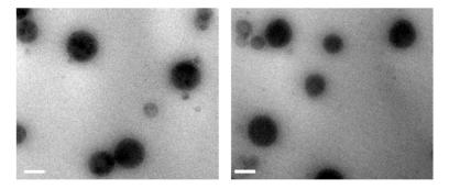
**Figure S2.** TEM image of DOX-PMs-1 (left) and DOX-PMs-3 (right) after incubation in PBS at pH 7.4 for 2 h. Mixed copolymers:DOX = 2:1, mass ratio. Scale bar, 100 nm.
