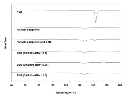
**Figure 2.** Differential scanning calorimeter patterns of CXB, physical mixture with excipients, physical mixture with excipients and CXB, and SDGs with different weight ratios of CXB/Cre-RH.
