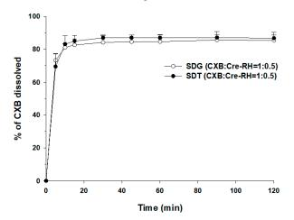
**Figure 4.** Dissolution profiles of CXB in pH 1.2 medium (sodium laurel sulfate (SLS) 0.5%) at 37.0  $\pm$  0.5 °C from SDG and SDT (*n* = 3).
