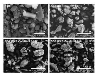
**Figure 1.** Scanning electron micrographs of CXB and solid dispersion granules (SDGs) with different weight ratios of CXB/Cre-RH. All the SDGs were 100–200 µm in size with irregular appearances.
